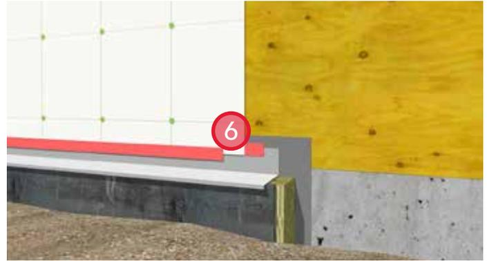
6. Install concrete protection board over insulation. Back fill dirt around the foundation wall.
