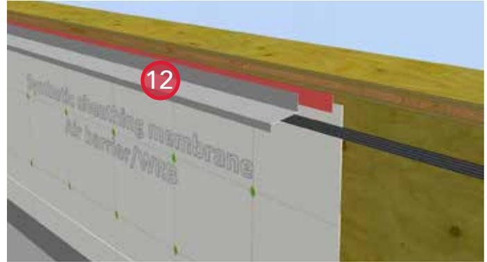
12. Install metal sub-flashing above parapet vent.
