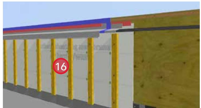
16. Install strapping and secure with recommended fasteners. Provide bugscreen at the top and bottom of the strapping and at the parapet vent.
