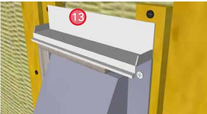
13. Install prefinished metal flashing above the vent hood trim.
