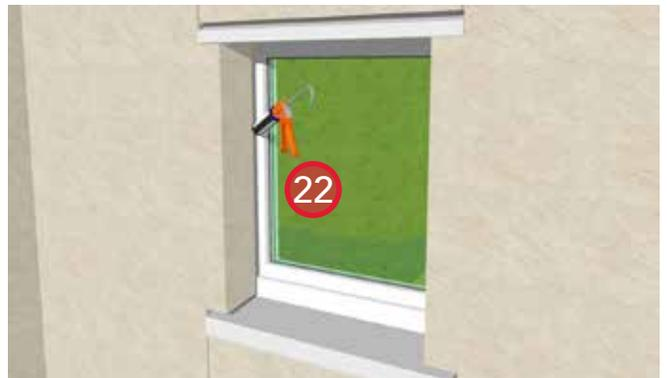
22. Install sealant around the perimeter of the window (top and sides) between the frame and stucco returns.
