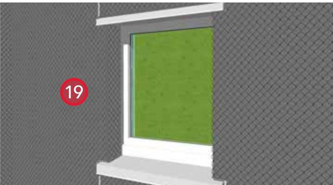
19. Secure stucco backer board and metal lath to the strapping. Secure backer board to blocking at jambs to support stucco returns.
