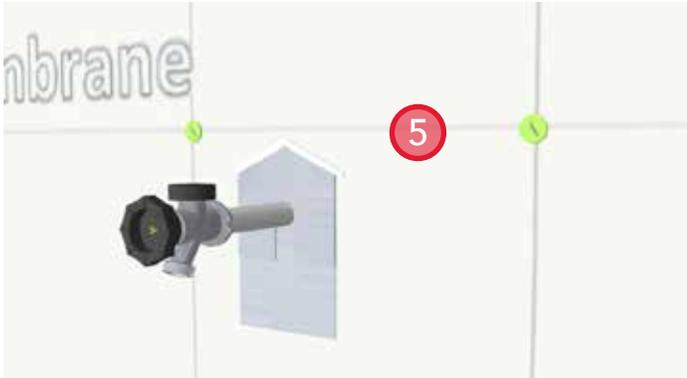
5. Install top sheet of foil-faced membrane. Positively lap the top sheet over the bottom sheet a minimum of 2".
