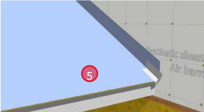
5. Install first step of the stepped flashing with a kickout to divert water towards the gutter and away from the adjacent wall.
