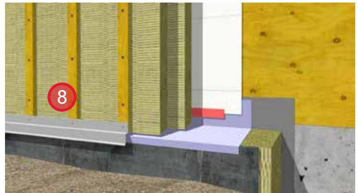
8. Install prefinished metal flashing to assist with water shedding.
