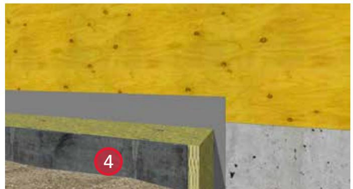
4. Install concrete protection board over insulation. Back fill dirt around the foundation wall.
