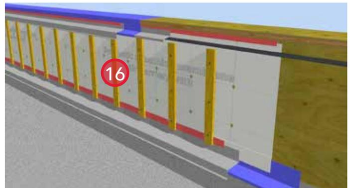
16. Install strapping. Ensure bugscreen is installed at the top and bottom of the strapping and at the parapet vent.
