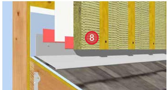
8. Install ROCKWOOL COMFORTBOARD™ and secure in place with strapping. Provide bugscreens at the top and bottom of the strapping.
