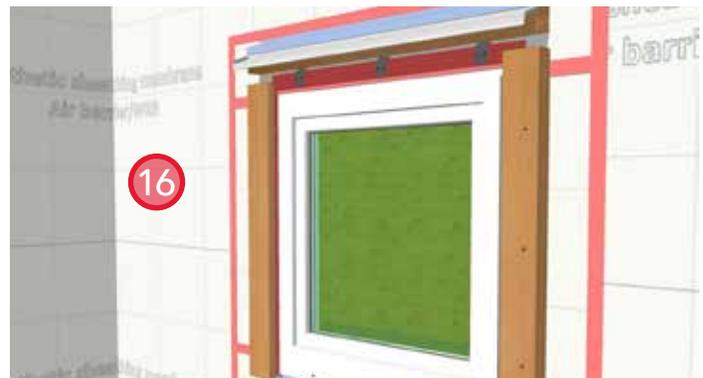
16. Install sheathing membrane. Ensure positive laps over all other layers. Seal all membrane laps with sheathing tape.
