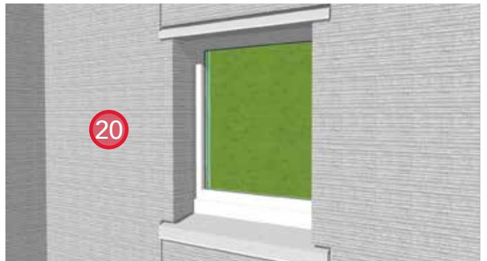
20. Install stucco scratch coat. Provide horizontal and vertical gaps (control joints) as necessary to account for differential movement between the wood framing and stucco cladding.
