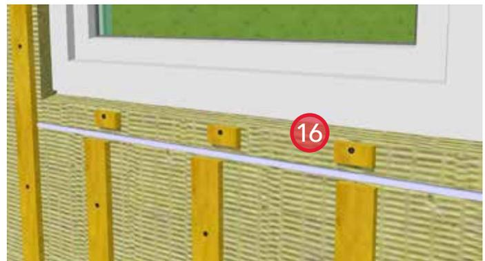
16. Install ROCKWOOL COMFORTBOARD™ above the self-adhered subsidiary sill membrane.
