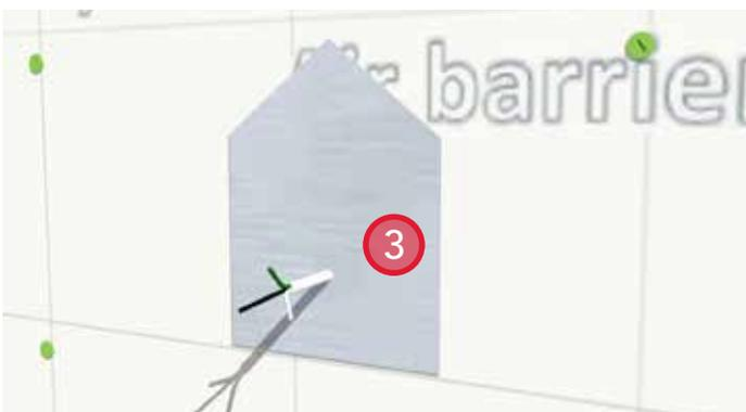
3. Pull the electrical wire through the wall and foil-faced, self-adhered membrane.
