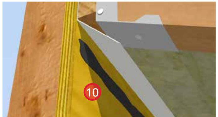
10. Apply a bead of sealant between the sheathing and sheathing membrane below the roof to increase air tightness.
