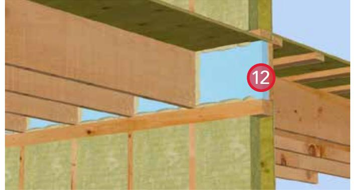
12. Install 2 lb. closed-cell spray or sealant around the perimeter of the rigid insulation to ensure air tightness and thermal barrier continuity.
