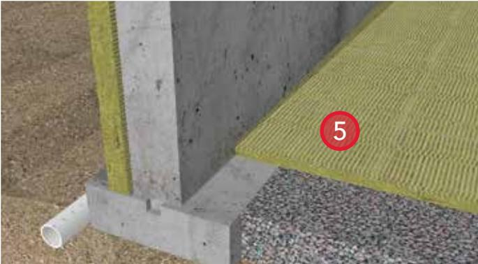
5. Install ROCKWOOL rigid board insulation at grade. Ensure the insulation is installed tight to the foundation wall.
