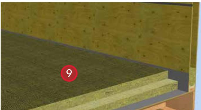
9. Install ROCKWOOL TOPROCK® DD as the bottom layer and TOPROCK® DD PLUS as the top layer.
