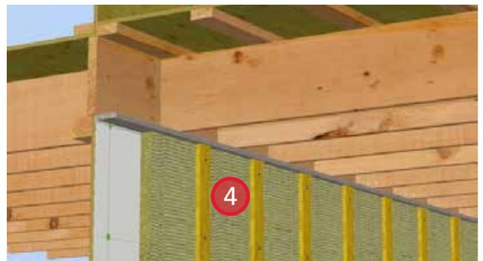
4. Install ROCKWOOL COMFORTBOARD™ and strapping with bugscreens, leaving a  $\frac{3}{4}$ " gap between the insulation and the top of the wall. Suggest using a 1x4 temporary spacer board to space the insulation.
