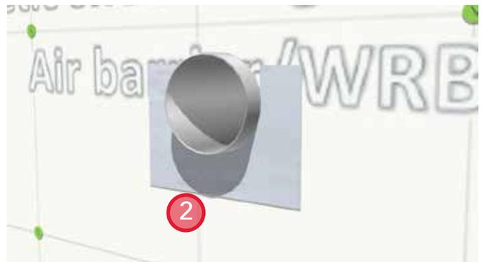
2. Install horseshoe-shaped self-adhered membrane below the exhaust vent.
