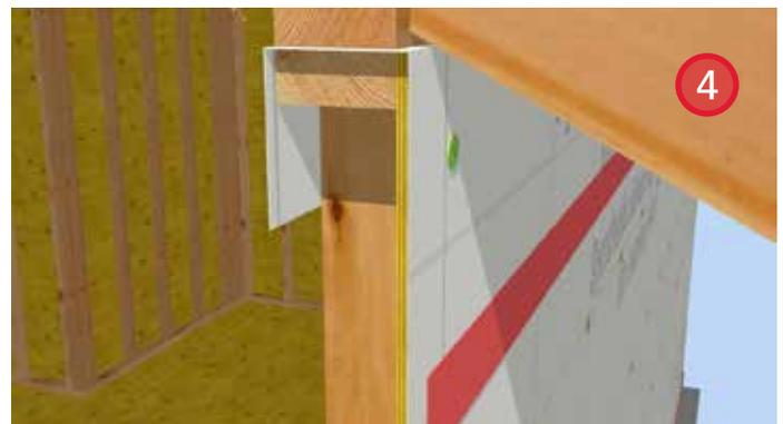
4. Seal the leading edge of the starter strip sheathing membrane with sheathing tape to maintain air barrier continuity.
