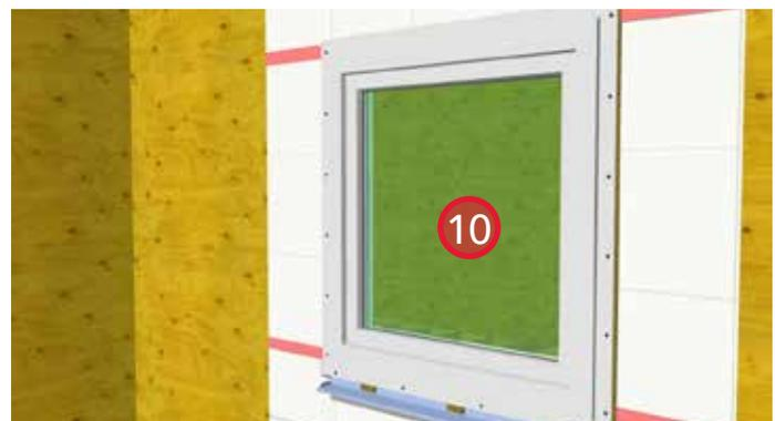
10. Install and structurally attach the window per manufacturer's specifications.
