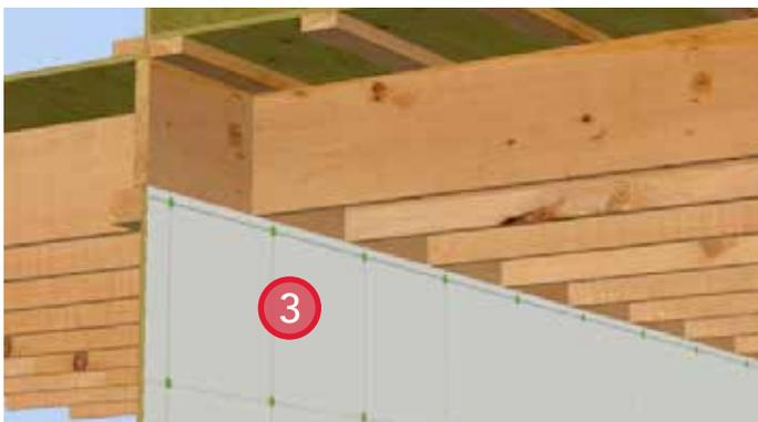
3. Install sheathing membrane and apply pressure to ensure adhesion to the sealant bead.
