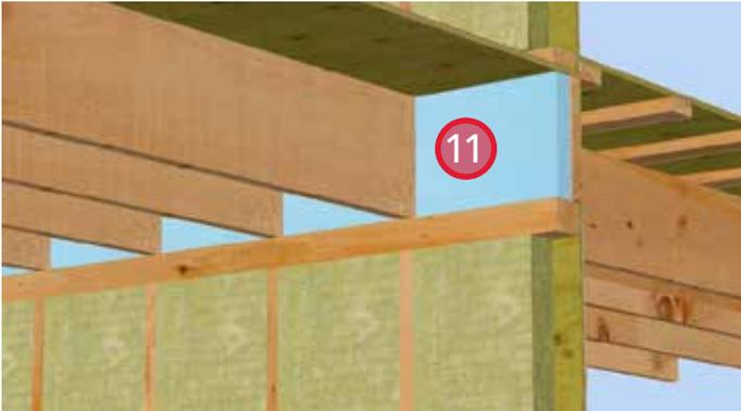
11. Install 3" rigid insulation in joist cavities. ROCKWOOL COMFORTBOARD™ and ROCKWOOL COMFORTBATT® can be used to meet thermal barrier protection requirements for foamed plastics.
