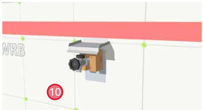
10. Install sheathing membrane and seal the leading edge with sheathing tape to maintain air barrier continuity. Ensure the membrane positively laps over other membranes and flashing.
