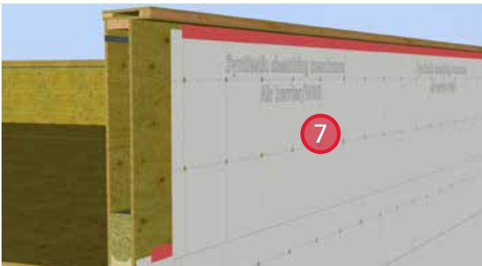
7. Install second layer of sheathing membrane and seal the leading edge with sheathing tape.
