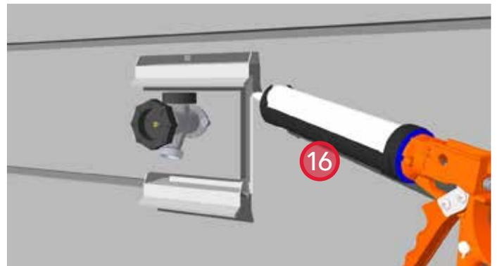
16. Apply sealant around the perimeter of the face plate and sill flashing (bottom and sides).
