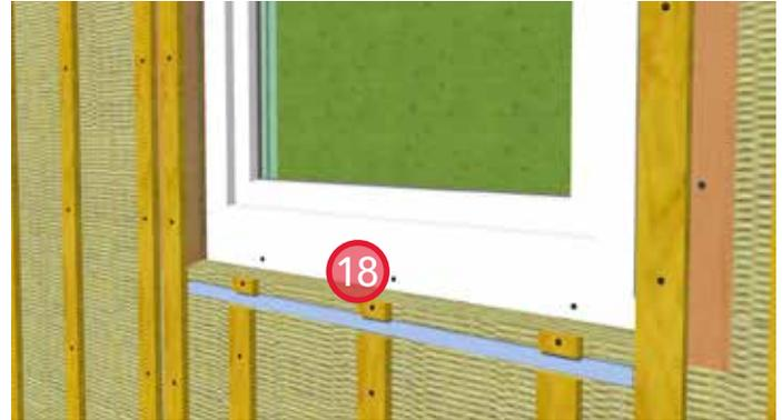
18. Install ROCKWOOL COMFORTBOARD™ above the self-adhered subsidiary sill membrane.
