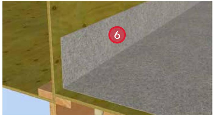
6. Install waterproof PVC balcony membrane and extend 8" up adjacent wall.
