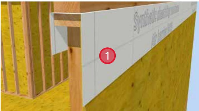
1. Install a starter strip of sheathing membrane between the top plates of the exterior walls. This will allow the air barrier to transition from the exterior sheathing membrane to the interior poly.
