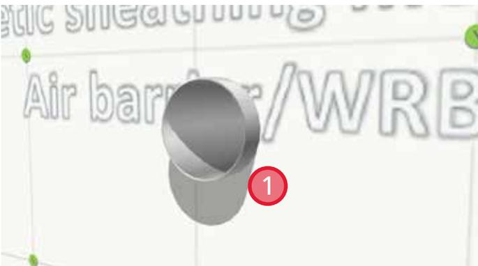
1. Install exhaust vent duct into an appropriately sized penetration in the sheathing and sheathing membrane. Place blocking/support on the interior side of the wall if required to secure the duct in place.
