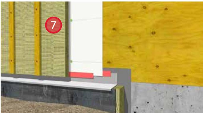
7. Install ROCKWOOL COMFORTBOARD™. Use strapping to hold the insulation; secure in place with recommended fasteners. Provide bugscreens at the top and bottom of the strapping.
