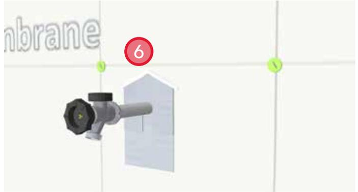
6. Apply mastic or other compatible sealant at the leading edge of the foil-faced membrane.
