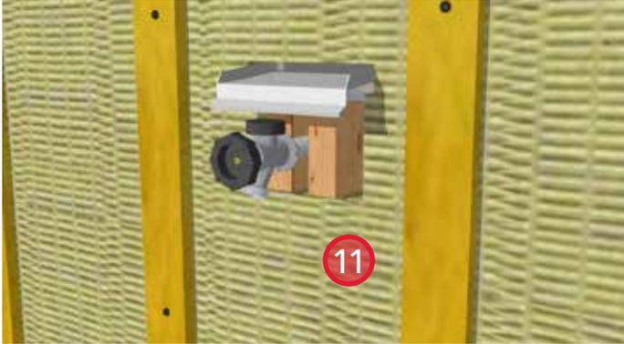
11. Install ROCKWOOL COMFORTBOARD™ and strapping. Provide bugscreens at the top and bottom of the strapping.
