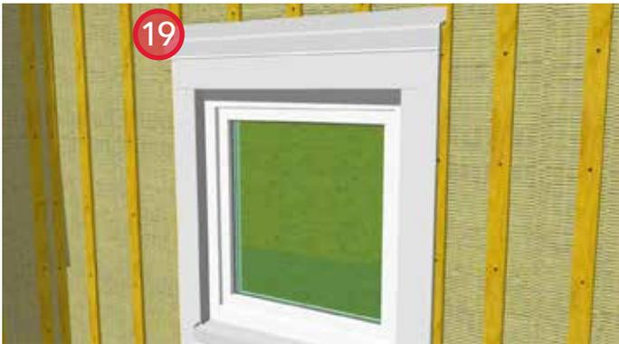
19. Install metal flashing to the strapping at the top window trim board to aid in water diversion.
