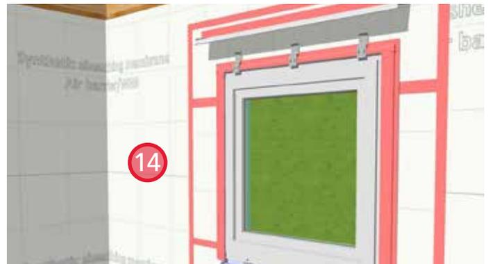
14. Install sheathing membrane. Ensure positive laps over all other layers. Seal all membrane laps with sheathing tape.
