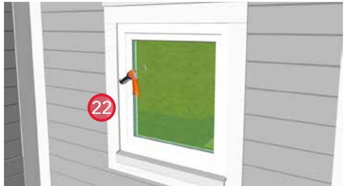
22. Apply sealant around the perimeter of the window (top and sides) between the frame and window trim boards.
