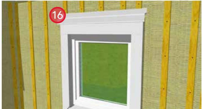
16. Install metal flashing to the strapping at the top window trim board to aid in water diversion.
