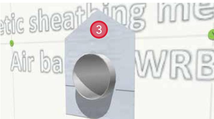
3. Install horseshoe-shaped self-adhered membrane above the exhaust vent. Taper the top of the membrane to facilitate water drainage.
