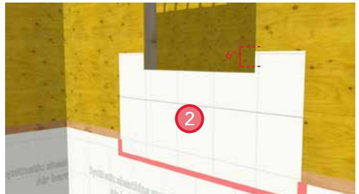
2. Install starter strip of sheathing membrane below the window rough opening. Seal the leading edges to the wall membrane below with sheathing tape.
