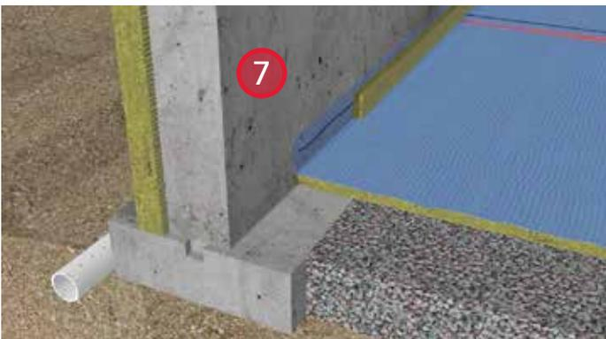
7. Install ROCKWOOL rigid board insulation in a strip the height of the slab along the base of the foundation wall. The insulation absorbs differential movement between the slab and foundation and provides a thermal break.
