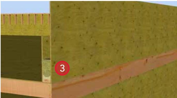
3. Install ROCKWOOL COMFORTBATT® insulation within the parapet to a height of the roof insulation as a minimum.
