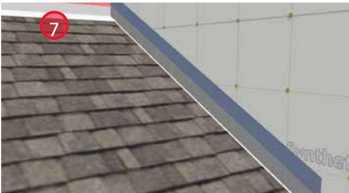
7. Install prefinished metal closure flashing on the above wall and seal the leading edge with sheathing tape.
