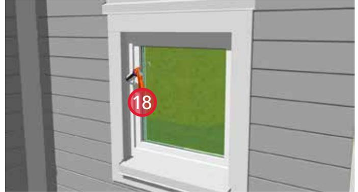
18. Install sealant around the perimeter of the window (top and sides) between the frame and window trim boards.
