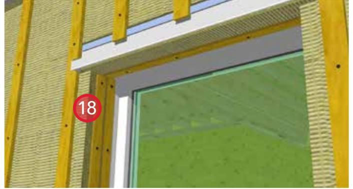
18. Install additional ROCKWOOL COMFORTBOARD™ at the jambs and head to over-insulate the window frame and secure with strapping fastened back to the blocking.
