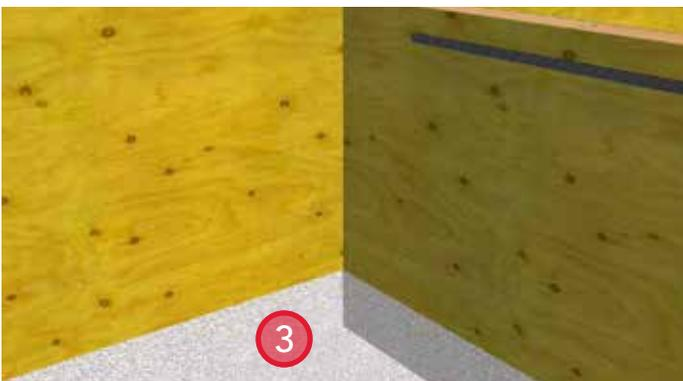
3. Install waterproof deck membrane. Return the deck membrane up the adjacent walls a minimum of 8".
