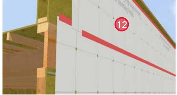
12. Install second layer of sheathing membrane and seal leading edges with sheathing tape.
