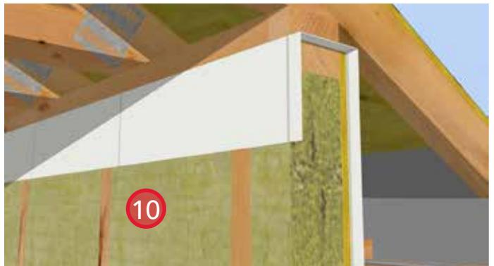
10. Install ROCKWOOL COMFORTBATT® within the interior stud cavities.
