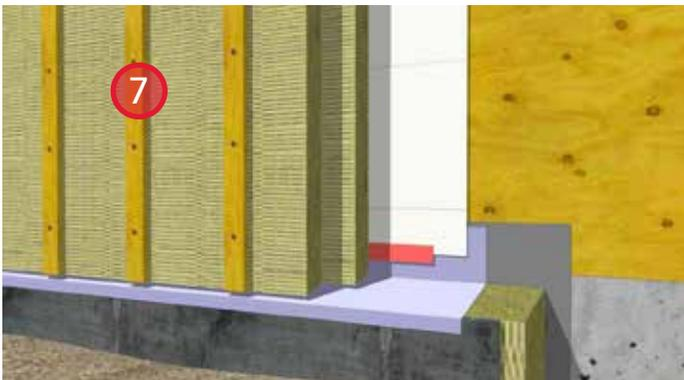
7. Install two layers of ROCKWOOL COMFORTBOARD™. Use strapping to hold the insulation and secure in place with recommended fasteners. Provide ugscreens at the top and bottom of the strapping.
