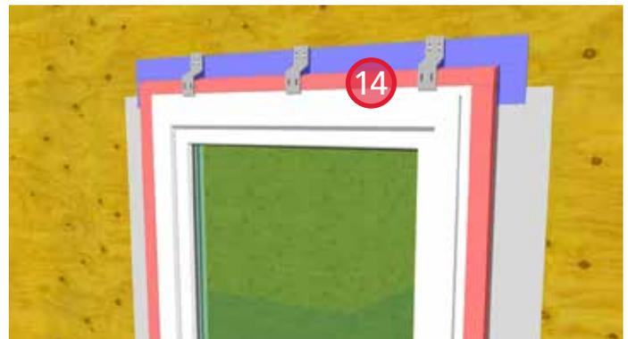
14. Install sheathing tape along the jambs and head of the window frame and extend onto the face of the wall. Install clips above the head flange to allow for shrinkage in the framing above the window opening.
