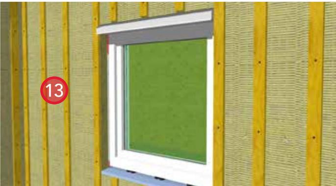
13. Install ROCKWOOL COMFORTBOARD™ and secure with strapping. Provide bugscreens at the top and bottom of the strapping.
