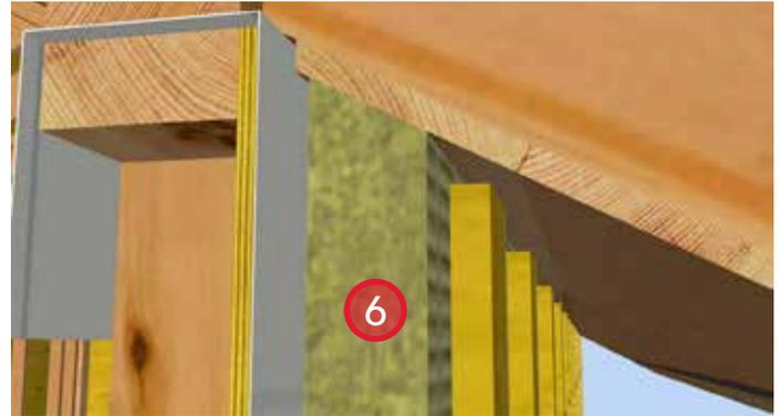
6. Install ROCKWOOL COMFORTBOARD™ and strapping to the exterior of the wall. Provide bugscreens at the top and bottom of the strapping.
