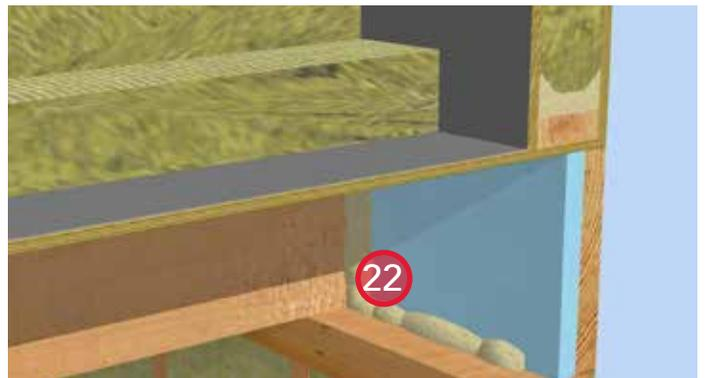
22. Install 2lb. closed-cell spray foam along the inside perimeter to maintain thermal barrier continuity.
