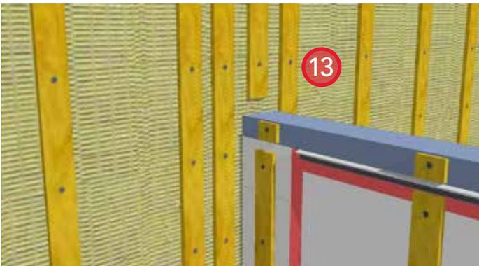
13. Install ROCKWOOL COMFORTBOARD™ and secure in place with strapping. Provide bugscreens at the top and bottom of the strapping.
