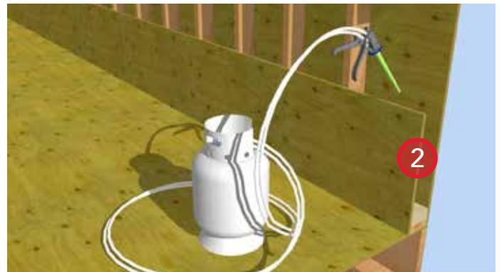
2. Install one 2" lift of 2 lb. closed-cell spray foam in the stud cavities of the parapet. Ensure the spray foam bonds to the sill plate and the sides of the parapet to complete the air barrier.
