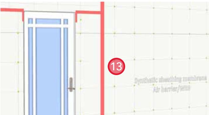
13. Install sheathing membrane to the rest of the wall. Seal the vertical leading edge with sheathing tape to maintain air barrier continuity.
