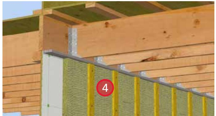
4. Install ROCKWOOL COMFORTBOARD™ and strapping with bugscreens, leaving a  $\frac{3}{4}$ " gap to ensure air barrier continuity through sheathing to rim joist interface. Suggest using a 1x4 temporary spacer board to space the insulation.
