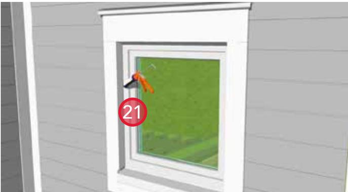
21. Apply sealant around the perimeter of the window (top and sides) between the frame and window trim boards.
