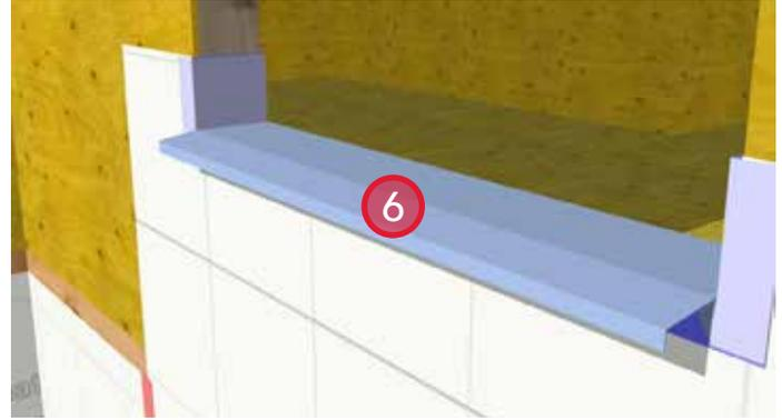
6. Install self-adhered subsidiary sill membrane to aid in water diversion over the ROCKWOOL COMFORTBOARD™. Leave the backer on the unsupported portion of the membrane until insulation is installed.
