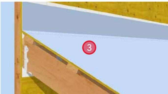
3. Install waterproof membrane. Extend the roof membrane 8" up the wall.
