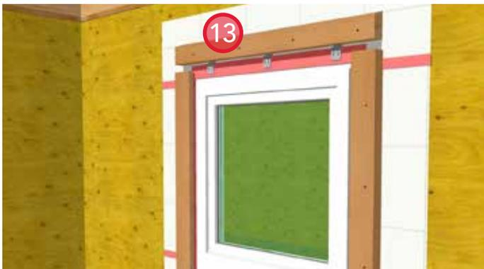
13. Install 2x4 blocking at jambs and head of window to support cultured stone trim. Taper the head blocking to provide slope for through wall flashing membrane.
