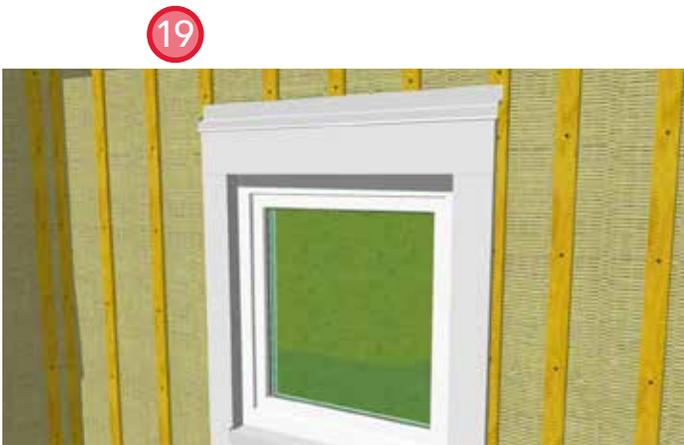
19. Install metal flashing to the strapping at the top window trim board to aid in water diversion.
