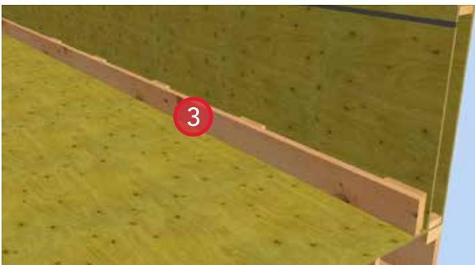
3. Install ventilation curb. Ensure the height of the curb is a minimum of 8" above the finished grade of the roof deck.
