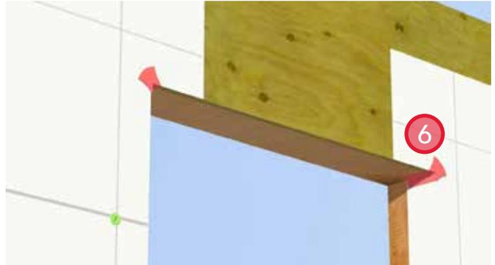
6. Install gussets constructed from sheathing tape at the upper corners of the rough opening.
