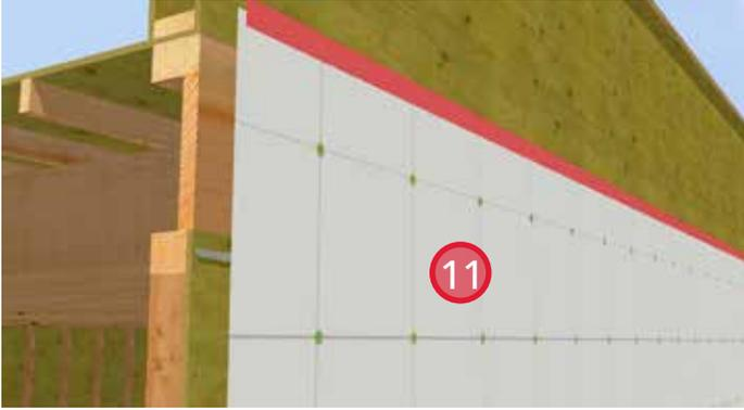
11. Install sheathing membrane and seal the leading edge with sheathing tape. Ensure pressure is applied to seal the sheathing membrane to the sealant bead.
