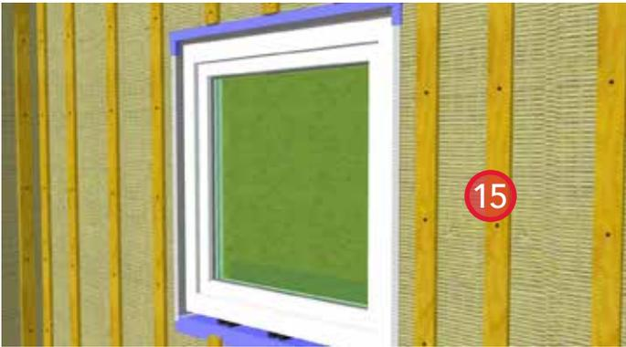
15. Install two layers of ROCKWOOL COMFORTBOARD™ and secure with strapping. Provide bugscreens at the top and bottom of the strapping.
