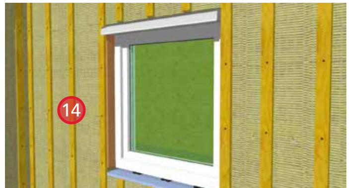
14. Install ROCKWOOL COMFORTBOARD™ and secure with strapping. Provide bugscreens at the top and bottom of the strapping.
