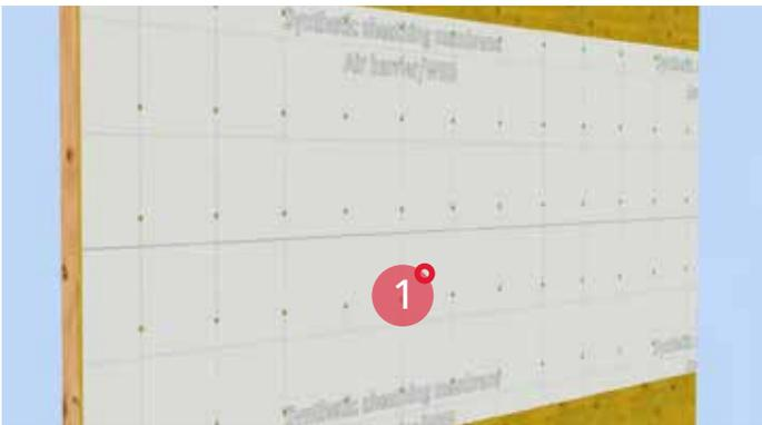
1. Install starter sheathing membrane under area where canopy will meet the wall.
