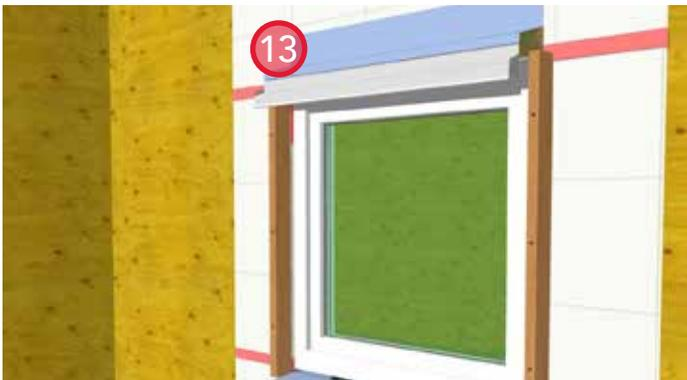
13. Install self-adhered membrane through wall flashing over the head blocking assembly and metal flashing back leg.
