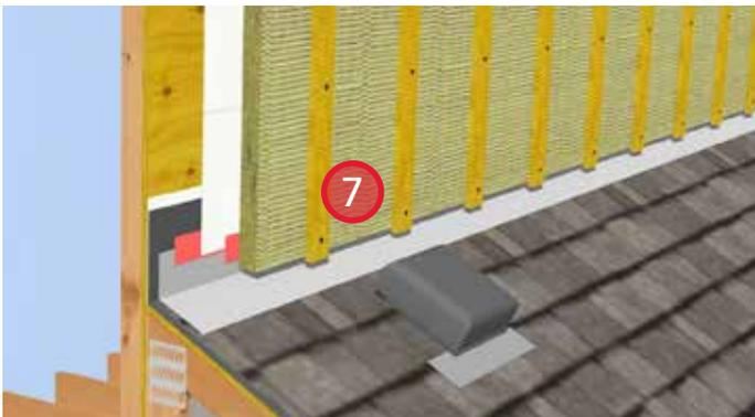
7. Install ROCKWOOL COMFORTBOARD™ and secure with strapping. Provide bugscreens at the top and bottom of the strapping.
