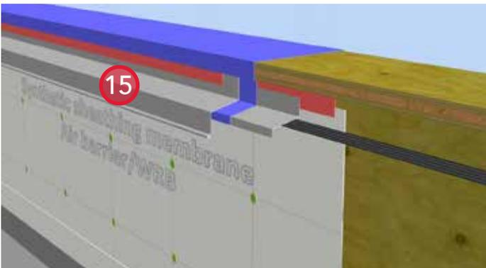
15. Install metal flashing and seal backleg with sheathing tape.
