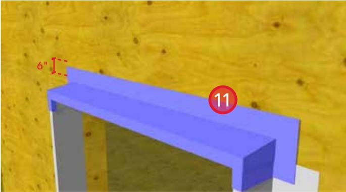
11. Install self-adhered membrane over the top of the plywood buck-out extending onto the plywood sheathing.
