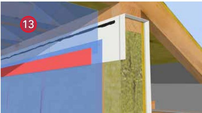
13. Install poly to the underside of the roof rafters and fasten with staples at the sealant bead to complete the air seal. Seal the leading edge of the poly with sheathing tape to maintain vapor barrier continuity.
