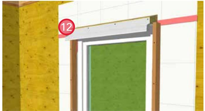
12. Install metal flashing to the head blocking assembly to aid in water diversion.
