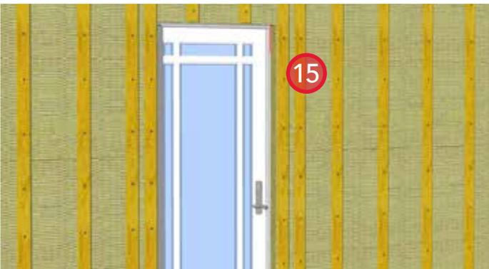
15. Install ROCKWOOL COMFORTBOARD™ and secure in place with strapping. Provide bugscreens at the bottom and top of the strapping.
