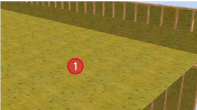
1. Typical conventional roof assembly construction. Parapet is partly framed to allow installation of insulation in the stud cavities.
