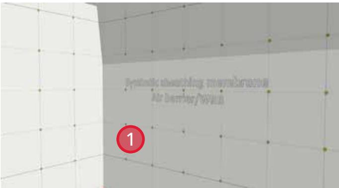
1. Install sheathing membrane at inside corner. Seal all laps with sheathing tape to maintain air barrier continuity.
