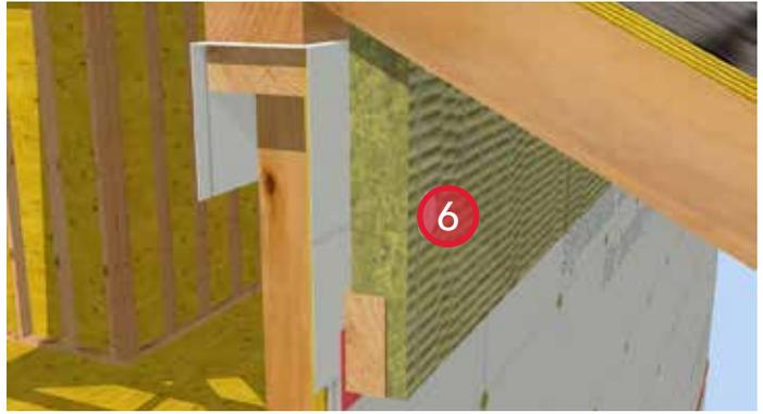
6. Install ROCKWOOL COMFORTBOARD™ and secure with recommended fasteners.
