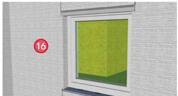
16. Install stucco scratch coat. Provide horizontal and vertical gaps (control joints) as necessary to account for differential movement between the wood framing and stucco cladding.
