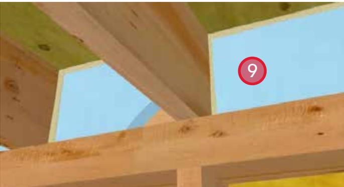
9. Install spray foam around the perimeter of the joist bay, sealing to the rigid insulation, top plate, joists and subfloor for air tightness and thermal barrier continuity.
