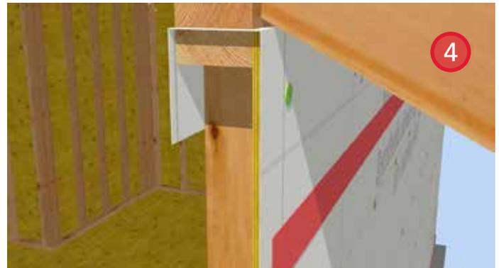
3. Install lower sheathing membrane. Make sure to lap under the starter strip.
