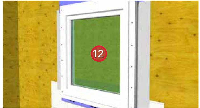
12. Install and structurally attach the window per manufacturer's specifications. Install 1/8" horseshoe shims behind sill flange to provide sub-sill drainage.
