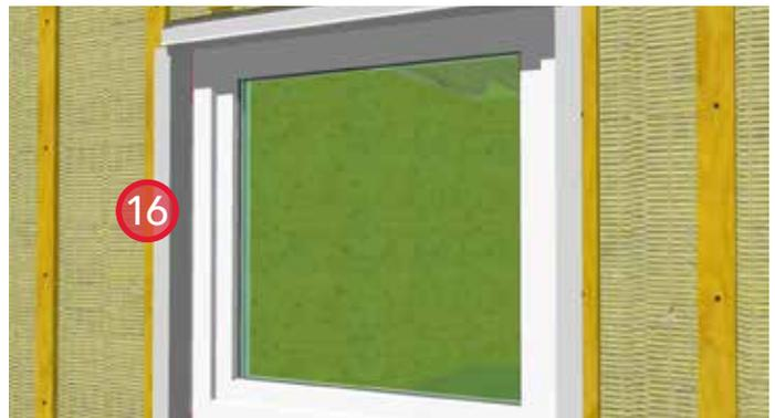
16. Install metal closure flashings at jambs to aid in water diversion. Flashing is supported by the wood strapping.
