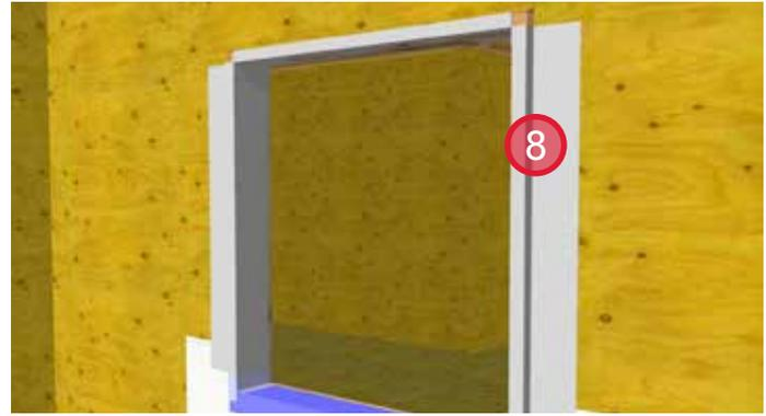
8. Wrap the buck-out jambs and window head with vapor permeable self-adhered membrane and positively lap over the membrane below.
