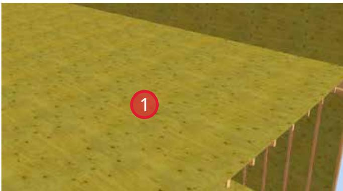
1. Typical vented roof assembly construction. Beveled strapping provides drainage slope.
