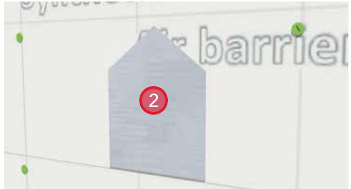
2. Install foil-faced, self-adhered membrane at the location of the electrical outlet.
