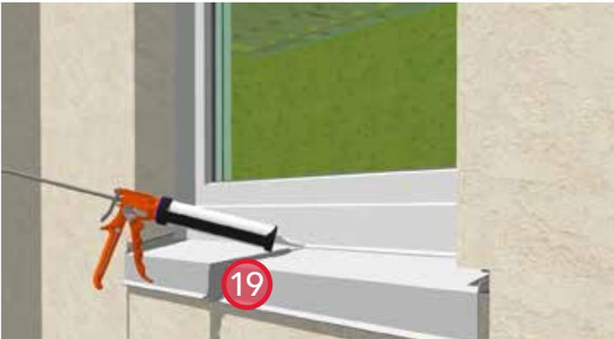
19. Apply sealant between the metal flashing and the window sill.
