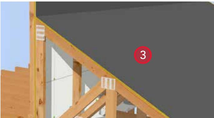
3. Install roof deck and waterproof membrane. Extend the waterproof membrane 8" up the wall.
