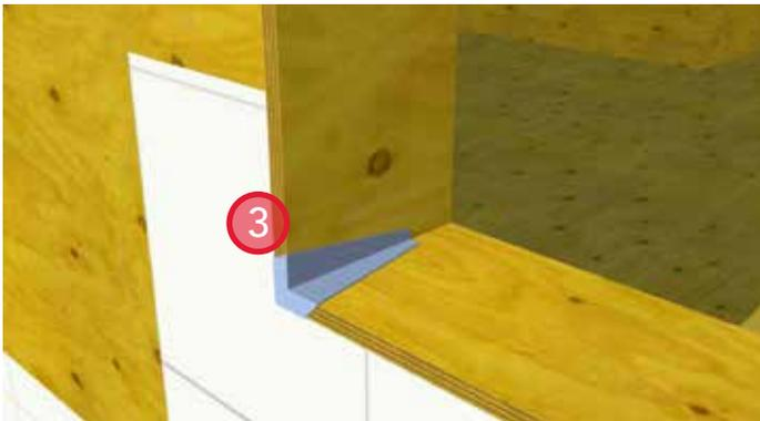
3. Install self-adhered membrane gussets at lower corners.
