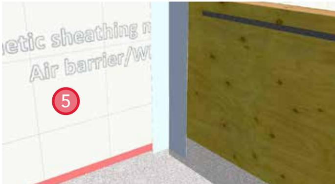
5. Install non-bitumious self-adhered membrane in the corner. Ensure the flashing adheres to the plywood on the guard wall and the adjacent sheathing membrane to provide for air barrier continuity.
