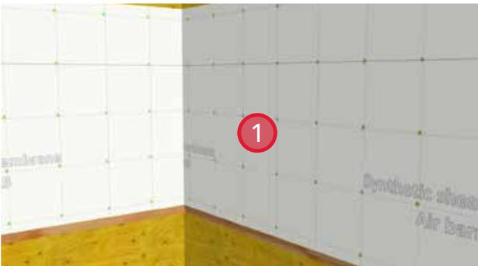
1. Install a starter strip of sheathing membrane that will extend beyond the framing of the roof.
