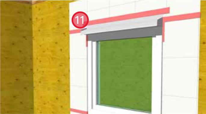
11. Install metal flashing at the head of the window. Seal the leading edge of the flashing with sheathing tape.
