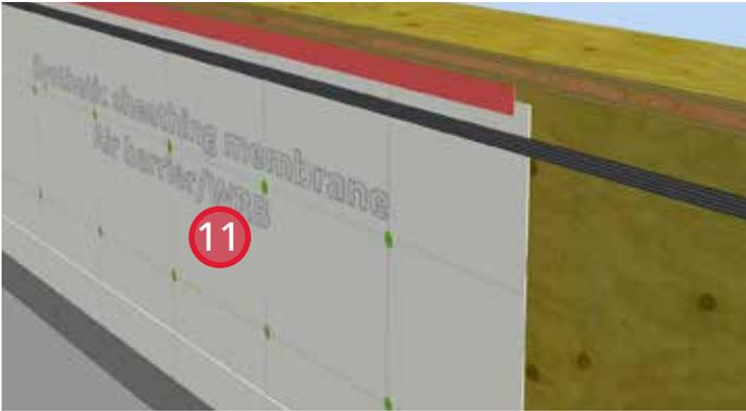
11. Install sheathing membrane as a water resistive barrier for the parapet. Seal the leading edge of the membrane with sheathing tape.
