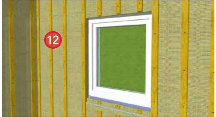
12. Install ROCKWOOL COMFORTBOARD™ and secure with strapping. Provide bugscreens at the top and bottom of the strapping.
