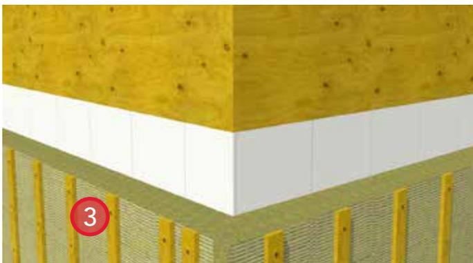
3. Install two layers of ROCKWOOL COMFORTBOARD™ below rim joist and taper top edge to drain. Use the strapping to support the insulation and secure in place with recommended fasteners. Provide bugscreens at the top and bottom of the strapping.
