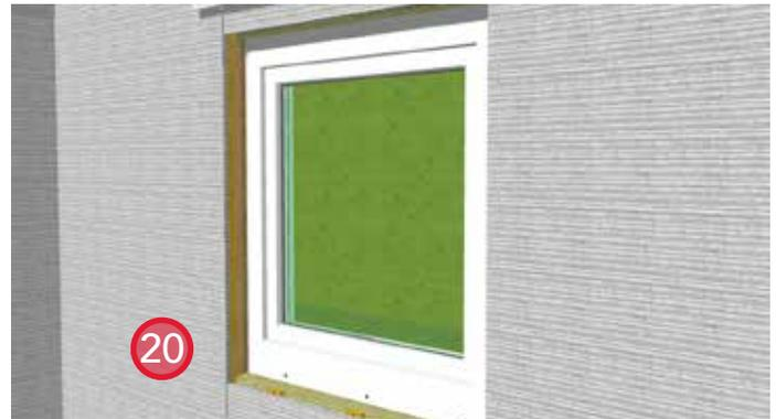
20. Install mortar scratch coat. Provide horizontal and vertical gaps (control joints) as necessary to account for differential movement between the wood framing and adhered masonry cladding.
