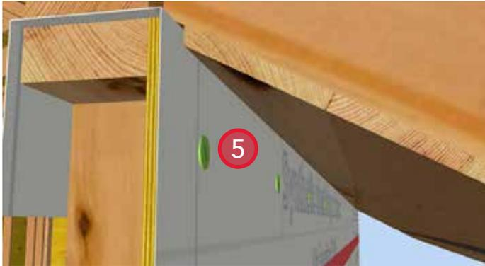
5. Install soffit material and vents.
