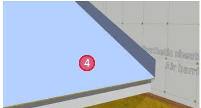
4. Install waterproof roof membrane. Return the membrane up the vertical face of the adjoining walls 1" beyond the projected back leg of the closure flashing.
