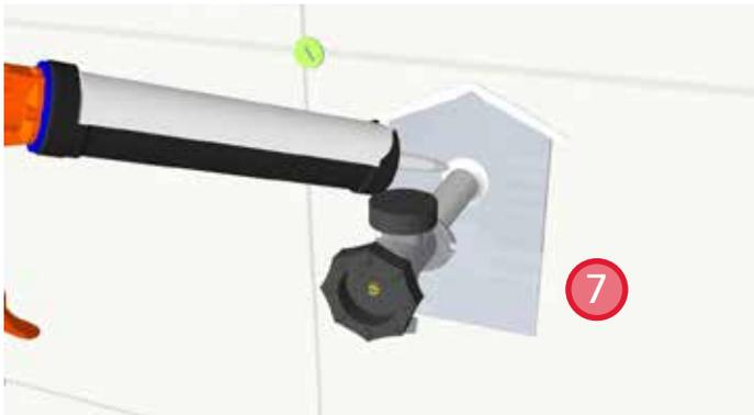
7. Apply a bead of sealant around the perimeter of the hose bib, ensuring good adhesion to the foil-faced membrane to maintain air barrier continuity.
