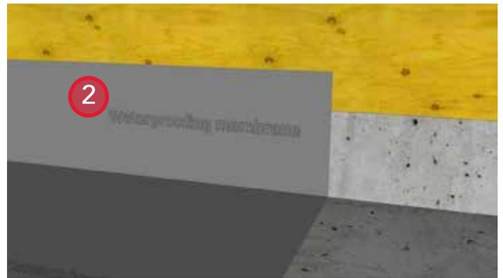
2. Install below-grade waterproofing membrane and extend a minimum 8" up adjacent wall. Provide a 2" overlap of waterproofing membrane onto the sheathing.
