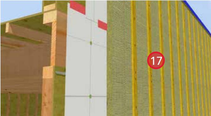
17. Install ROCKWOOL COMFORTBOARD™ and secure with strapping.
