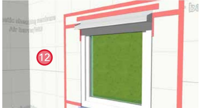
12. Install sheathing membrane. Ensure positive laps over all other layers. Seal all membrane laps with sheathing tape.
