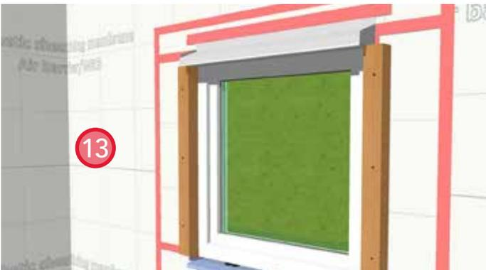
13. Install sheathing membrane. Ensure positive laps over all other layers. Seal all membrane laps with sheathing tape.
