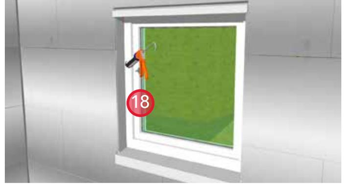
18. Install sealant around the perimeter of the window (top and sides) between the frame and metal closure flashings.
