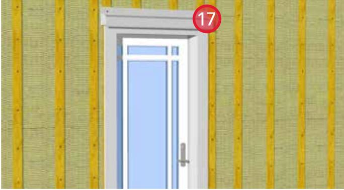
17. Install metal flashing to the strapping above the top trim board to aid in water diversion.
