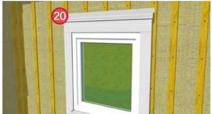
20. Install metal flashing to the strapping over the top window trim board.
