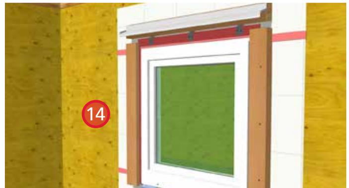
14. Install metal flashing to the head blocking to aid in water diversion.
