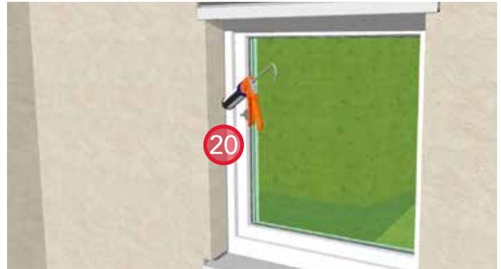
20. Install sealant around the perimeter of the window (top and sides) between the frame and stucco returns.
