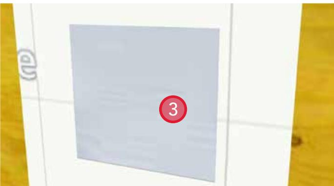
3. Install a backing of self-adhered membrane over the starter sheathing membrane. Install sealant at the top and sides of the self-adhered membrane.
