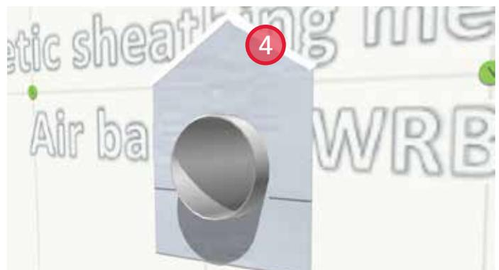
4. Seal the leading edge of the foil-faced membrane with mastic or another compatible sealant.
