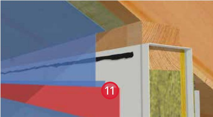
11. Install the poly sheet to the underside of the roof rafters. Fasten the poly sheet to the sheathing membrane with staples at the sealant bead to complete the air seal and seal the leading edge with sheathing tape.
