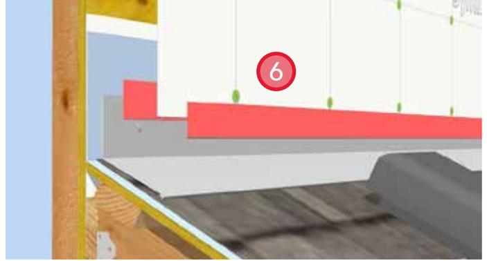
6. Install sheathing membrane and lap over the metal flashing. Seal the leading edge with sheathing tape to complete air barrier transition.
