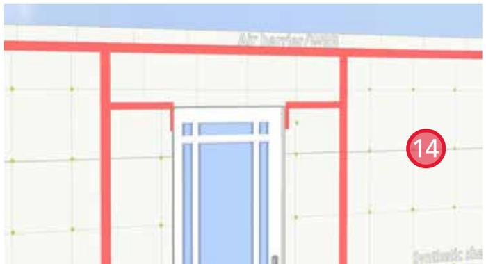
14. Install sheathing membrane from above and seal the leading edge with sheathing tape to maintain air barrier continuity. Ensure the sheathing membrane laps over membrane layers below.
