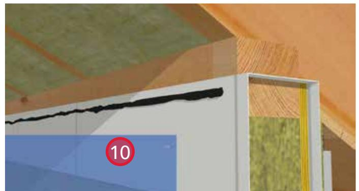
10. Install a bead of acoustical sealant on the sheathing membrane at the lower top plate to transition the air barrier from the wall to the ceiling.
