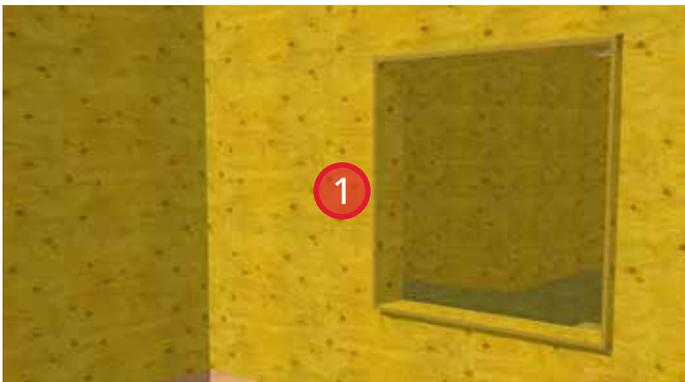
1. Typical wood frame construction at sheathing stage with 3/4" plywood window buck. The window buck depth should match the thickness of the installed insulation. Install sloped window head at top of buck-out.
