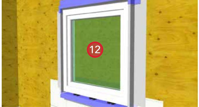
12. Install and structurally attach the window per manufacturer's specifications. Position the window at the front of the buck-out in order to minimize thermal bridging effects.
