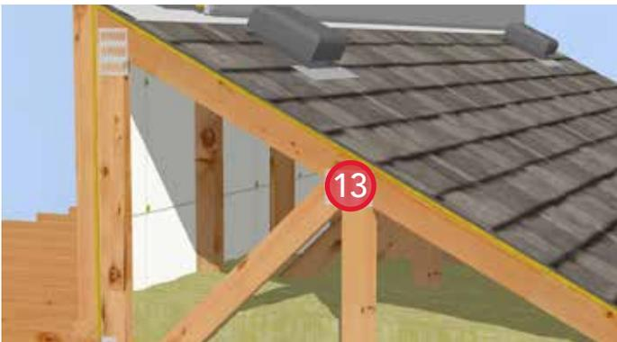
13. Install ROCKWOOL COMFORTBATT® in the attic space. Insulate wall adjoining attic space and occupied space with COMFORTBATT®.
