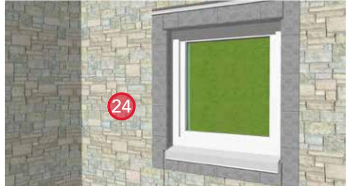
18. Adhere cultured stone cladding with mortar bond coat. Grout stone cladding joints to maintain continuity of the water shedding surface.
