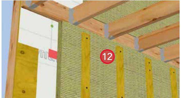
12. Install ROCKWOOL COMFORTBOARD™ and secure in place with strapping. Provide bugscreens at the top and bottom of the strapping.
