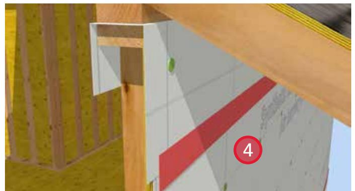
4. Install sheathing tape at the leading edge of the sheathing membrane to complete air barrier continuity.
