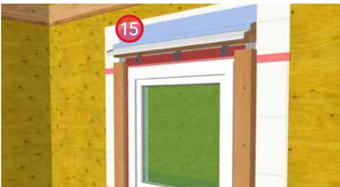
15. Install self-adhered membrane through wall flashing over the head blocking and metal flashing back leg.
