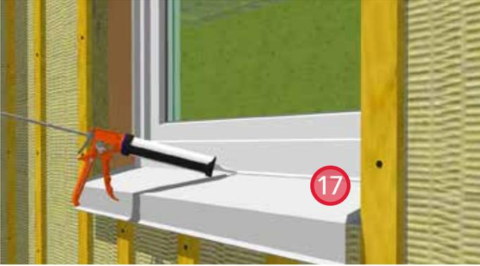
17. Apply sealant between the metal flashing and the window sill. Install stucco cladding. Secure stucco returns to blocking at the jambs.
