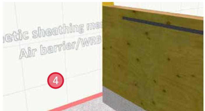
4. Install sheathing membrane to the above grade wall. Seal the leading edges to the deck membrane with sealant and sheathing tape to maintain air barrier continuity.
