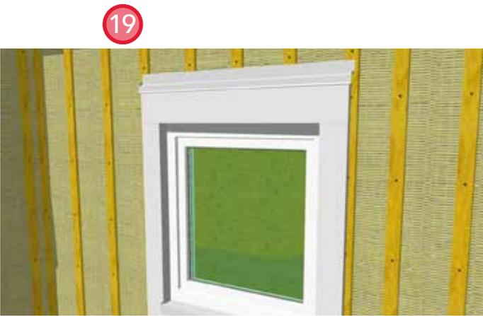
19. Install metal flashing to the strapping at the top window trim board to aid in water diversion.
