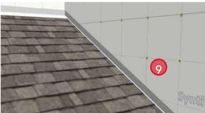
9. Install sheathing membrane. Ensure it laps over the prefinished metal closure flashing.
