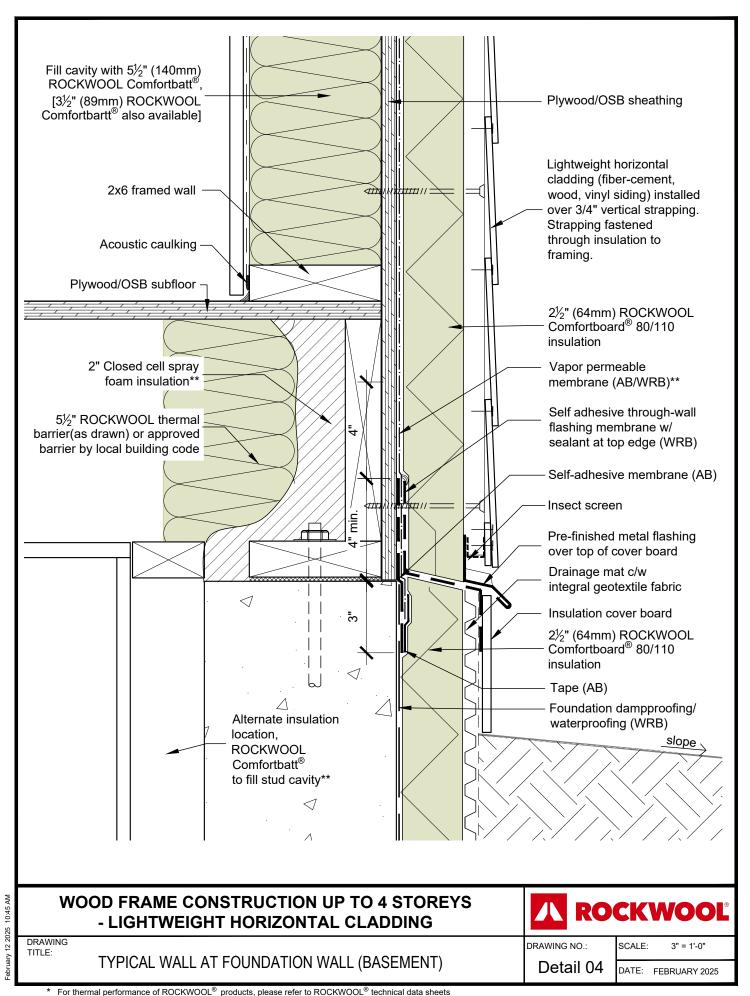
\*\* Interior vapor control for cold climates shown. For further climate zone specific considerations for thermal, air and vapor control methodologies and requirements, please contact ROCKWOOL<sup>TM</sup> Building Science.
