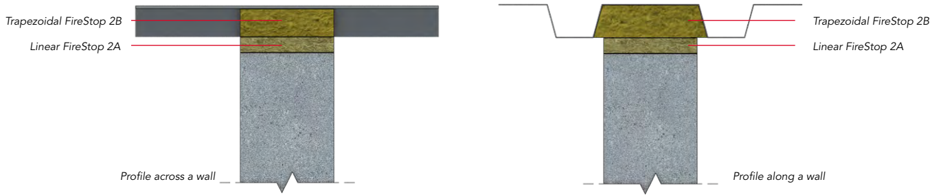
Figure 4 Profiled metal deck over blockwork wall
