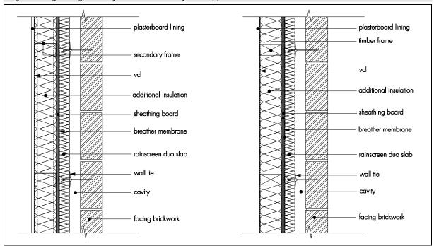
15.5 The insulation should be installed to coincide with the steel/timber frame, with retaining discs used in conjunction with the wall ties at no more than 600 mm horizontally and 450 mm vertically.
