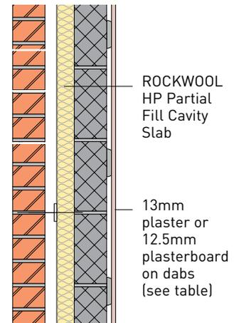
General Notes: The U-values assume that walls are lined with plasterboard on dab or 13mm lightweight plaster (lambda 0.220). Block sizes assumed to be 440x215mm, mortar joints assumed to be 10mm wide, stainless steel wall ties with a cross-sectional area of 12.5mm<sup>2</sup> for cavities up to 170mm wide. Above 170mm, the cross sectional area of tie wires is assumed to be 25mm<sup>2</sup>.
