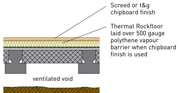
The standard thickness of ROCKWOOL Thermal Rockfloor range from 50mm-100mm. For thickness greater than 100mm we recommend double layering the product. Please contact our ROCKWOOL Technical solutions dept. for U-values relating to a specific project or application.
