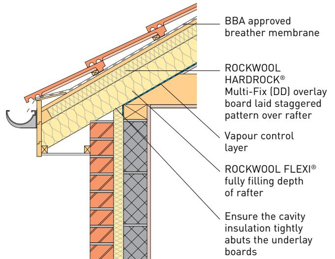
The Rockfall system is totally fire safe, minimises thermal bridging and provides an effective acoustic barrier against external noise pollution. The system comprises of a high density ROCKWOOL HARDROCK® Multi-Fix (DD) board mechanically fixed over the rafters with ROCKWOOL FLEXI® fitted between rafters. An air tight VCL membrane is stapled to the underside of the rafters finished with 12.5mm plasterboard.
