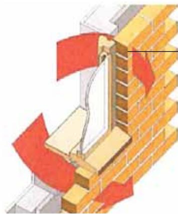
Thermal bridging at door and window reveals can result in 20% heat loss from buildings if left un-insulated.
