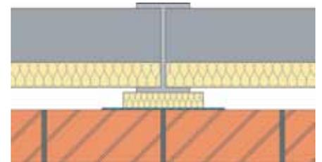
Plan view on column intrusion into cavity
