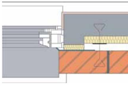
Plan view at jamb ROCKCLOSE® with Aluminium frame in rebated 'check' reveal
