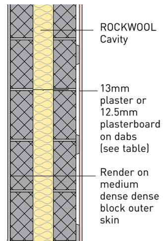
General Notes: The U-values assume that walls are lined with plasterboard on dab or 13mm lightweight plaster (lambda 0.220). Block sizes assumed to be 440 x 215mm, mortar joints assumed to be 10mm wide, stainless steel wall ties with a cross-sectional area of 12.5mm<sup>2</sup> for cavities up to 170mm wide. Above 170mm, the cross sectional area of tie wires is assumed to be 25mm<sup>2</sup>.
