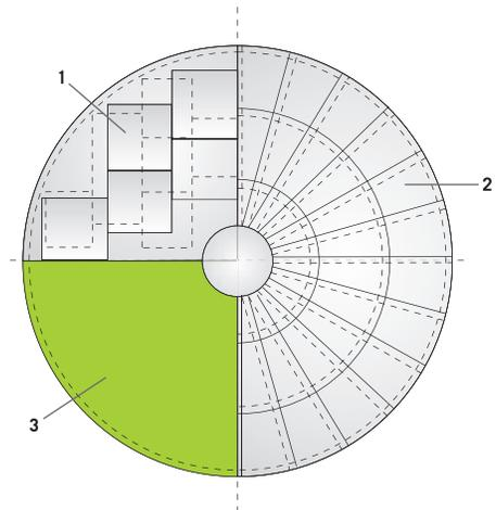
1. Finishing with aluminum cladding - 2. Finishing with steel radial segments - 3. ProRox® insulation
