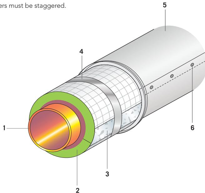
1. Pipe - 2. Insulation: ProRox® MA 960<sup>NA</sup> - 3. Self-adhesive aluminum tape - 4. Steel bands - 5. Sheet cladding - 6. Sheet-metal screw or rivet
