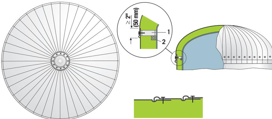
1. Supporting construction - 2. Mounting support
