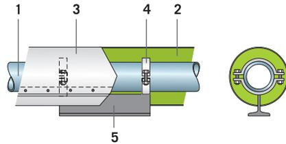
1. Pipe - 2. Insulation: ProRox® PS 960<sup>NA</sup> – pipe section - 3. Sheet cladding - 4. Pipe clamp - 5. Pipe saddle
