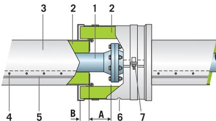
1. Pipe - 2. ProRox® insulation - 3. Cladding - 4. Sheet-metal screw or rivet - 5. Swage - 6. Drainage opening - 7. Straps –  $B \geq 2"$  (50 mm) - A = Bolt length + 1.2" (30 mm)
