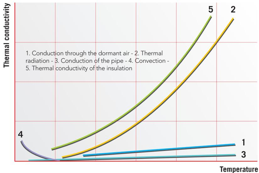
Thermal conductivities for industrial/mechanical insulation can be measured according to the test methods below.
