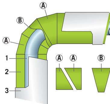
1. Pipe - 2. Insulation: ProRox® Pipe Sections - 3. Cladding - A and B = Segmented pipe sections
