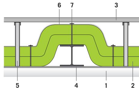
1. Duct wall - 2. ProRox® insulation - 3. Metal cladding: corrugated sheet - 4. Reinforcing element - 5. Supporting construction and spacer - 6. Aluminum foil (optional) - 7. Welding pins/clips
