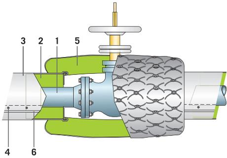
1. Pipe - 2. Insulation: ProRox® Pipe Sections - 3. Cladding - 4. Sheet-metal screw or rivet - 5. Removable coverings (insulated from the inside) - 6. Swage
