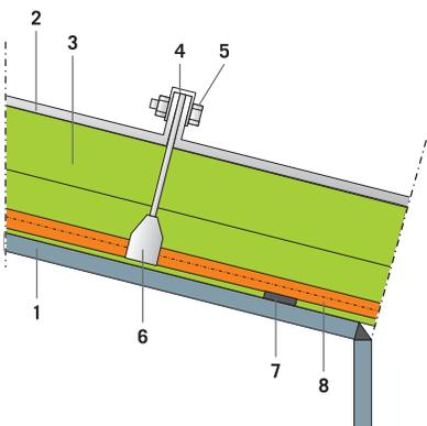
1. Tank roof - 2. Cladding - 3. ProRox® pressure resistant insulation - 4. Aluminum finishing strip - 5. Bolts and rivets (stainless steel) - 6. Strip (stainless steel) - 7. Weld - 8. Welded steel bar
