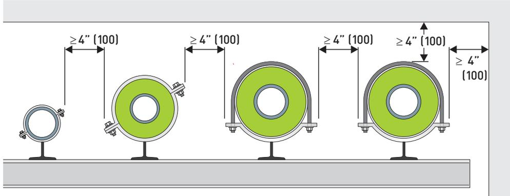
Minimum distances within range of pipe flanges; dimensions in inches (mm)
