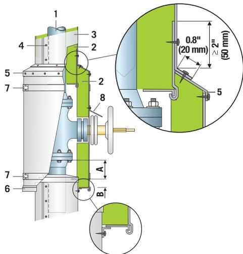
1. Pipe - 2. ProRox® insulation - 3. Cladding - 4. Sheet-metal screw or rivet - 5. Rain deflector - 6. Lock washer - 7. Straps - 8. Rain deflector -
