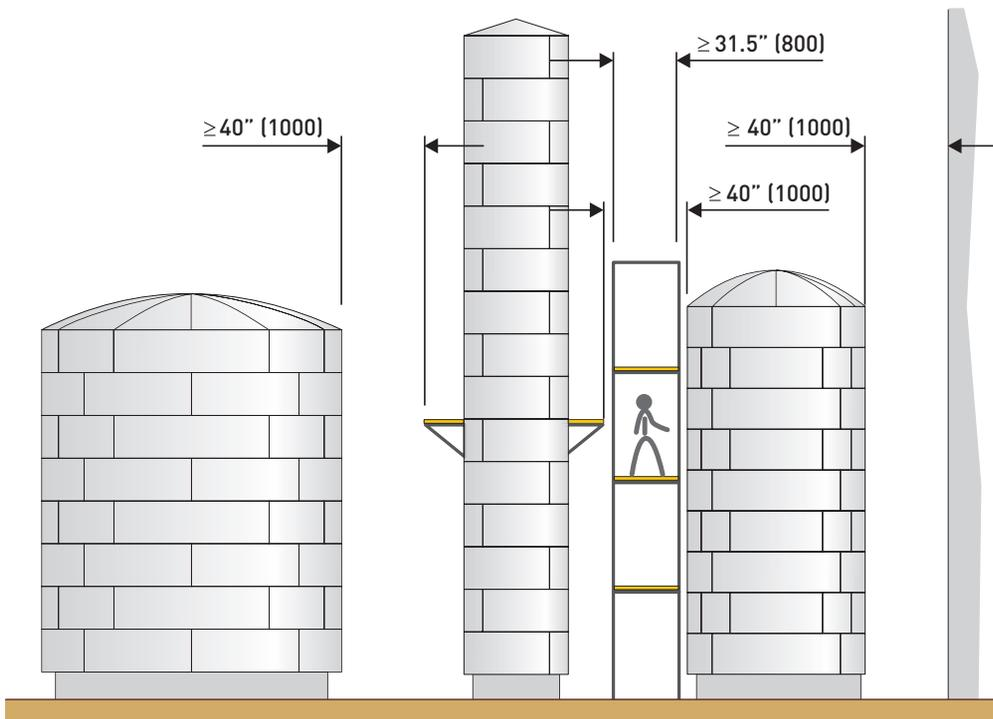
Minimum distances between insulated pipes; dimensions in inches (mm)
