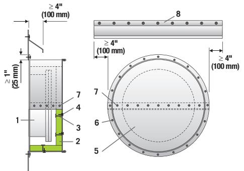
1. Manhole - 2. ProRox® insulation - 3. Stiffener - 4. Stiffener screw or rivet - 5. End cap - 6. Mounting rim - 7. Sheet-metal screw or rivet - 8. Rain deflector
