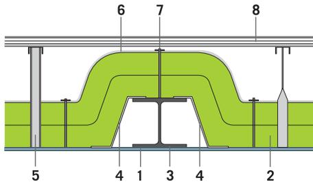
1. Duct wall - 2. ProRox® insulation - 3. Reinforcing element - 4. Covering sheet - 5. Support construction and spacer - 6. Aluminum foil (optional) - 7. Welding pins/clips - 8. Metal cladding: corrugated sheet
