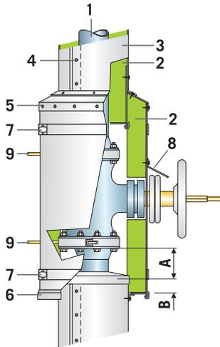
1. Pipe - 2. ProRox® insulation - 3. Cladding - 4. Sheet-metal screw or rivet - 5. Collar - 6. Collar - 7. Clamps - 8. Rain deflector - 9. Leak detection fitting -  $B \geq 2"$  (50 mm) -  $A = \text{bolt length} + 1.2"$  (30 mm)
