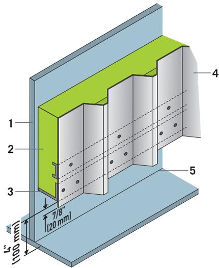
1. Tank wall - 2. ProRox® insulation - 3. Support ring - 4. Cladding - 5. Welded seam
