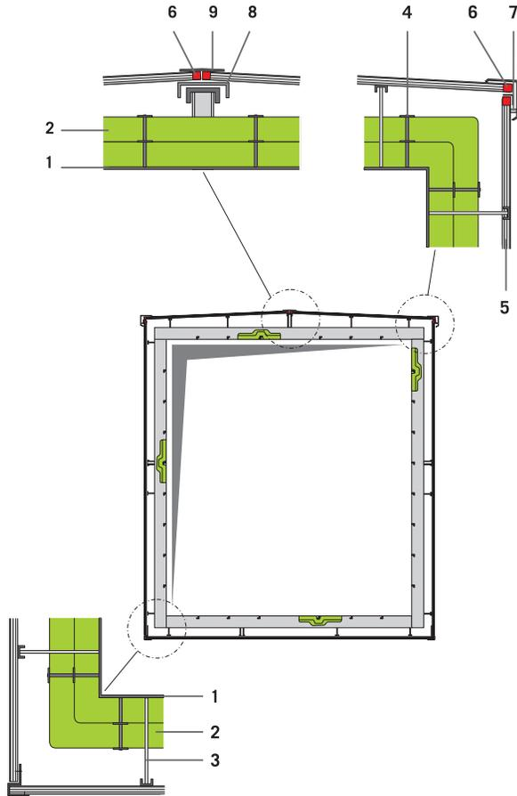
1. Duct wall - 2. ProRox® insulation - 3. Support construction and spacer - 4. Welding pins/clips - 5. Metal cladding: corrugated sheet - 6. Extension (trapezoid) - 7. Z-shaped spacer - 8. Support construction - 9. Ridge
