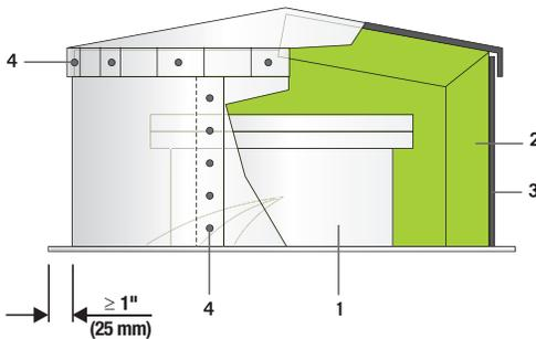
1. Manhole - 2. ProRox® insulation - 3. Cladding - 4. Sheet-metal screw
