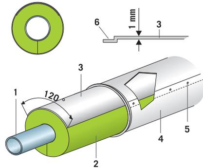
1. Pipe - 2. Insulation: ProRox® PS 980<sup>NA</sup> Pipe Sections - 3. Reinforcement sheet (may not be required) - 4. Cladding - 5. Sheet-metal screw or rivet - 6. Joggle
