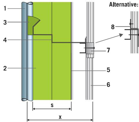
1. Boiler wall - 2. ProRox® insulation - 3. Fill with loose rock wool - 4. Convection barrier sheet - 5. Aluminum foil if required - 6. Metal cladding - 7. MF profile filling - 8. Z-profile separating sheet
