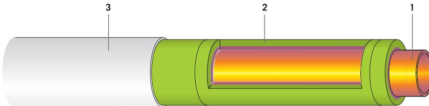
1. Pipe - 2. Insulation: ProRox® Pipe Sections or Pipe Wraps (Mats): ProRox® MA 960<sup>NA</sup> - 3. Cladding
