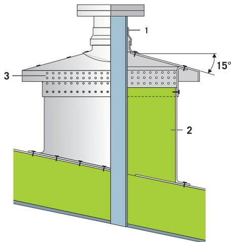
1. Sealing tape - 2. ProRox® insulation - 3. Perforated sheet (ventilation)
