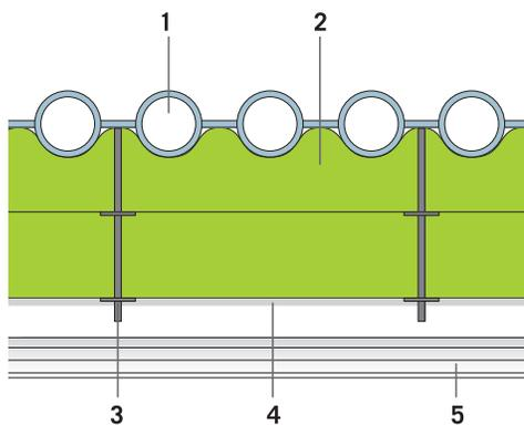
1. Finned pipe - 2. ProRox® insulation - 3. Fastening pins with spring plates - 4. Aluminum foil if necessary -
