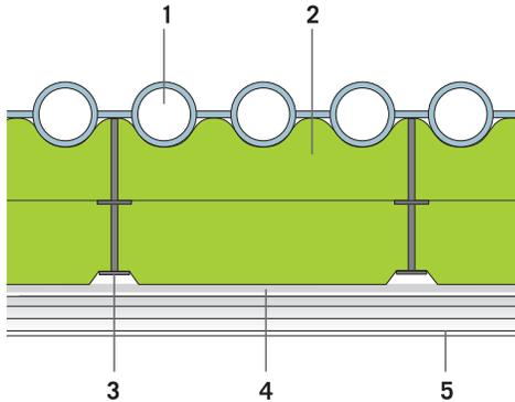
1. Tube wall - 2. ProRox® insulation – 3. spring plates - 4. Aluminum foil if required - 5. Cladding (e.g. profiled sheet)
