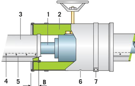
1. Pipe - 2. ProRox® insulation - 3. Cladding - 4. Sheet-metal screw or rivet - 5. Swage - 6. Drainage opening - 7. Straps –  $B \geq 2"$  (50 mm)
