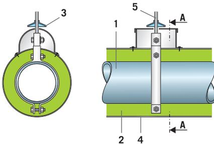
1. Pipe - 2. Insulation: ProRox® Pipe Sections - 3. Collar - 4. Sheet cladding - 5. Pipe hanger
