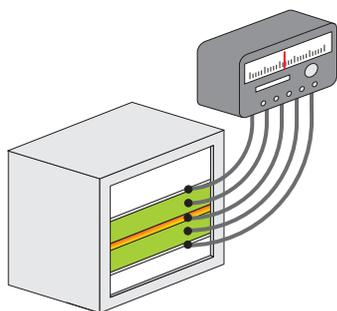
The core components of the apparatus usually consist of two cold-surface units and a guarded hot-surface unit. The insulation material to be measured is sandwiched between these units. The thermal conductivity is calculated at the mean temperature between the hot and the cold side and expressed at the hot face temperature.
