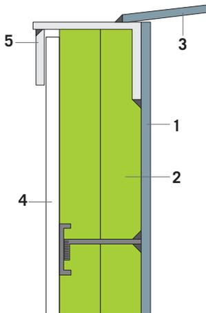
1. Tank wall - 2. ProRox® insulation - 3. Tank roof - 4. Cladding (aluminum) - 5. Deflector
