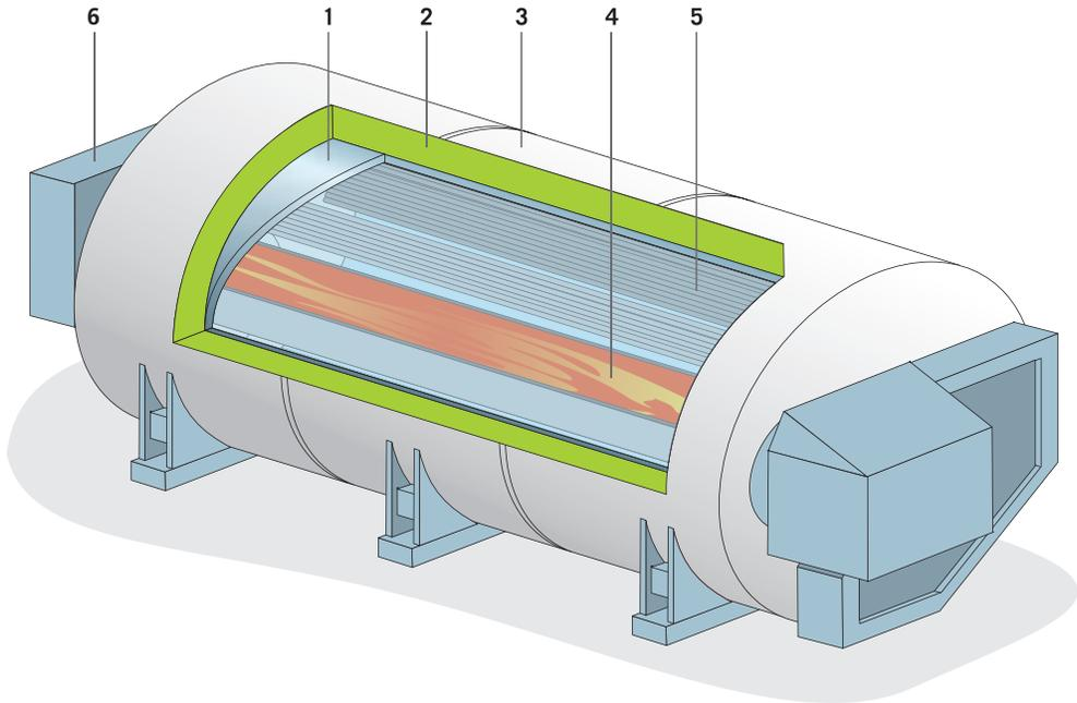
1. Boiler casing - 2. ProRox® insulation - 3. Cladding - 4. Flame tube - 5. Fire tube - 6. Reversing chamber
