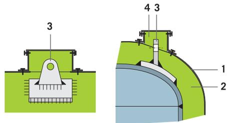
1. Cladding - 2. ProRox® insulation - 3. Crane hooks - 4. Insulation covering for the crane hook
