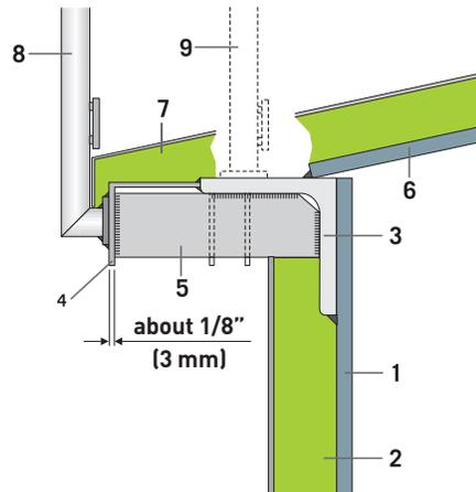
1. Tank wall - 2. ProRox® insulation - 3. L-profile - 4. Rain deflector - 5. Support strip - 6. Tank top - 7. Insulation: ProRox® pressure resistant insulation - 8. Railing - 9. Not insulated roof
