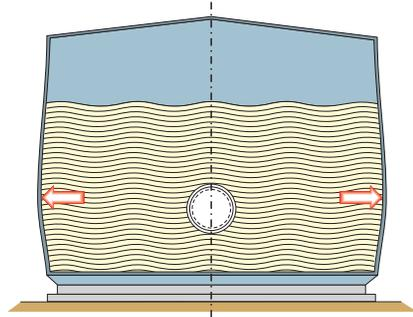
the tank diameter. Example: The diameter of a storage tank -  $\varnothing$  65 ft (20 m), Avg T 430 °F (220 °C) - will increase approx. 2 1/2" (60 mm). This consequently increases the tank circumference by approx. 7" (180 mm). To avoid stress/tension on the insulation protection (aluminum sheeting) selecting flexible ProRox® insulation board (slab) or wrap (mat) is important. For high temperatures, anticipate further expansion by fitting profiled sheeting.
