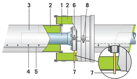
1. Pipe - 2. ProRox® insulation - 3. Cladding - 4. Sheet-metal screw or rivet - 5. Swage - 6. Flange band - 7. Leak detection fitting - 8. Clamps
