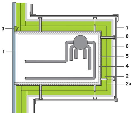
1. Boiler wall - 2. ProRox® insulation - 3. Fill up with loose fill stone wool (mineral wool) - 4. Support construction - 5. Dead space sheeting - 6. Aluminum foil if required - 7. Metal cladding/Preformed sheets - 8. Support construction and spacer
