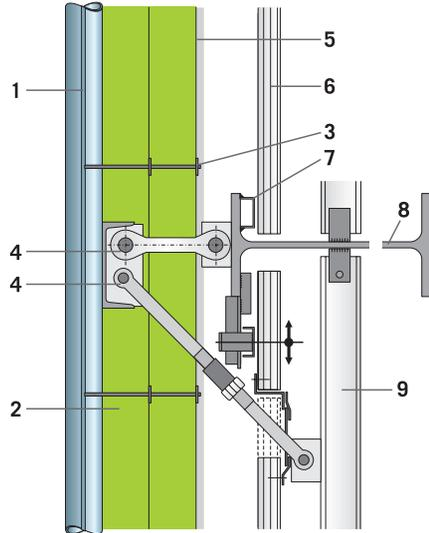
1. Boiler wall - ProRox® insulation - 3. Mat pins with clips - 4. Buckstay deflectors - 5. Aluminum foil if required - 6. Metal cladding/profiled sheet - 7. Substructure - 8. Cold buckstay - 9. Boiler handle
