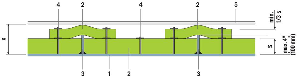
1. Duct wall - 2. ProRox® insulation - 3. Reinforcing ribs - 4. Welding pins with clips - 5. Metal cladding
