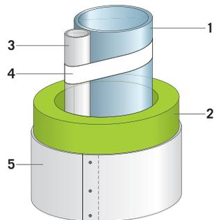
1. Pipe - 2. Insulation: ProRox® Pipe Sections -
