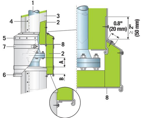
1. Pipe - 2. ProRox® insulation - 3. Sheet - 4. Sheet-metal screw or rivet - 5. Rain deflector - 6. Lock washer - 7. Straps - 8. Lock washer -  $B \geq 2"$  (50 mm) - A = Screw length + 1.2" (30 mm)
