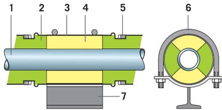
1. Pipe - 2. Insulation: ProRox® PS 960<sup>NA</sup> pipe sections - 3. Sheet cladding - 4. Load-bearing insulation - 5. Seal - 6. Stirrup - 7. Pipe saddle
