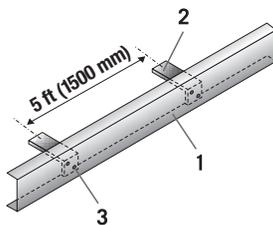
1. Horizontal support ring - 2. Spacer - 3. Fixing
