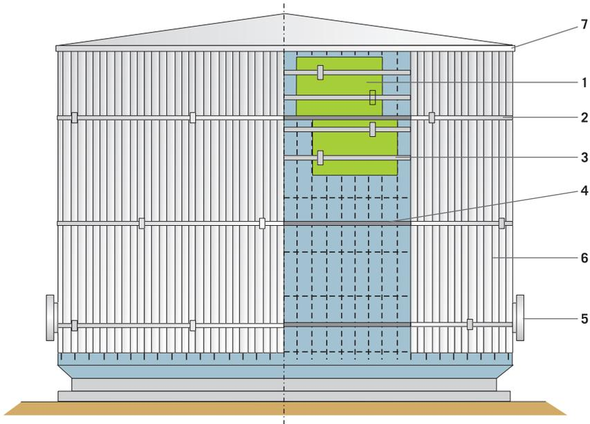
1. ProRox® insulation - 2. Stainless steel bands (weather proofing) - 3. Stainless steel bands - 4. Support ring - 5. Protrusion - 6. Cladding - 7. Roof/wall connection
