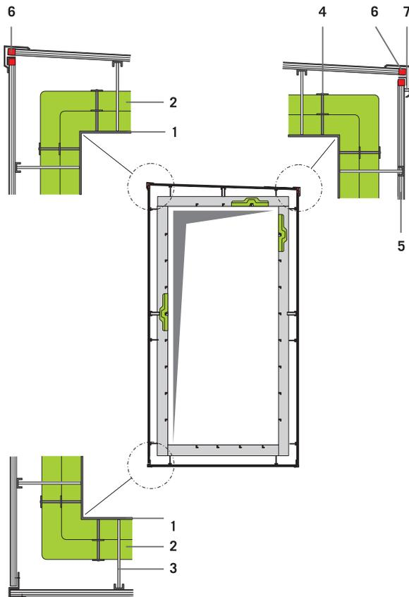
1. Duct wall - 2. ProRox® insulation - 3. Support construction and spacer - 4. Welding pins/clips - 5. Metal cladding; corrugated sheet - 6. Extension (trapezoid) - 7. Z-shaped spacer
