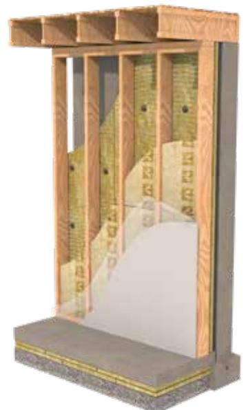
The combination of ROCKWOOL Comfortboard® 80 and ROCKWOOL Comfortbatt® ensures optimum long-term thermal performance from basement wall assembly.
