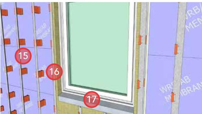
17. Tie in the sub-sill drainage membrane, ensuring that it is positively sloped and fully supported by the ROCKWOOL CAVITYROCK®.
