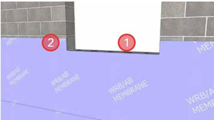
This installation is for an aluminum window frame (non-curtain wall) in punched configuration. Detail could be modified slightly based on window type.
