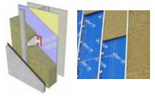
Thermally isolated galvanized steel clip attached to wall with screws through plastic isolation pad.
