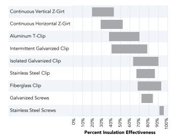
This same information can also be used to help select an appropriate thickness of ROCKWOOL CAVITYROCK<sup>®</sup> insulation over an uninsulated 3 5/8" steel stud frame back-up wall in the chart below. For example, to get to an effective R-20 with this back-up wall, 6" of CAVITYROCK<sup>®</sup> insulation is required with several different cladding support systems.
