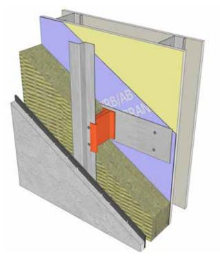
Example of the use of galvanized sheet steel strips to provide structural backer for cladding support clips away from studs.
