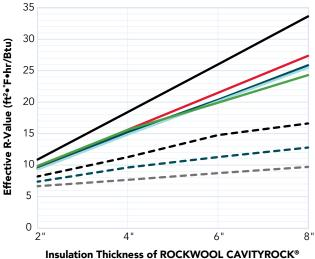
Insulation Thickness of ROCKWOOL CAVITYROCK® Over Empty 3 5/8" Steel Stud Back-up Wall
