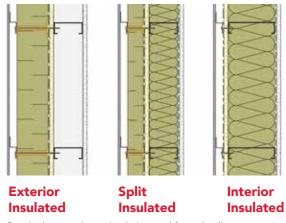
Standard approaches to insulating steel-framed wall assemblies, referred to as exterior insulated, split insulated and interior insulated depending on the placement of insulation.
