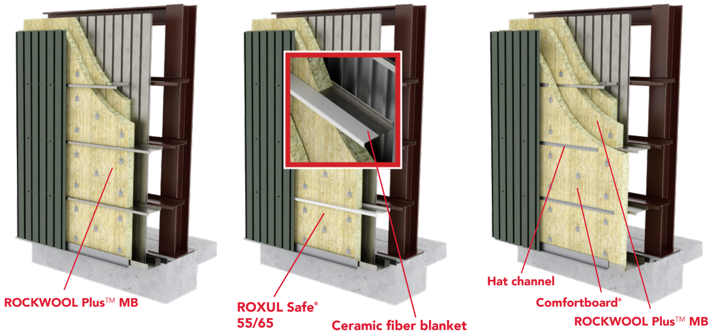
Assembly 3: Exterior wall with no fire-resistance requirement but high thermal performance desired. An extra layer of continuous insulation (c.i.) is added over the horizontal girts, with hat channels fastened through the c.i.
