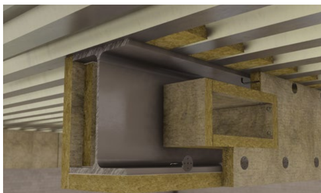
Figure 10 Beam with square or rectangular holes (boxed protection - dry joints)
