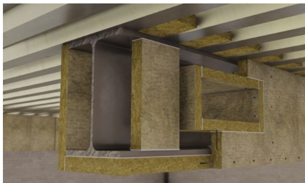
Figure 8 Beam with square or rectangular holes (boxed protection - glued and pinned joints)
