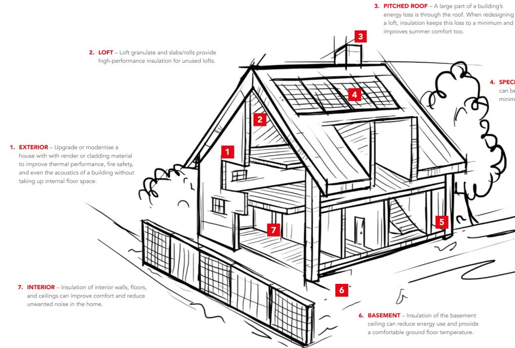
4. SPECIALISED SOLUTIONS - Special insulation can be incorporated under solar systems to minimise heat loss and increase energy efficiency.
