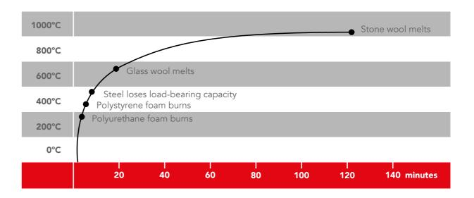
Behaviour of different materials according to the standard time/temperature curve of fire resistance standard ISO 834. Physical damage occurs.
