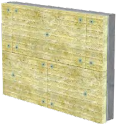
Figure 14. Illustration showing an example of a minimum of five attachments per board
