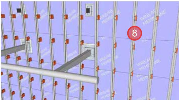
8. Secure clip and rail cladding attachment system to the concrete block wall per the manufacturer's specifications. Refer to the front end of this guide for further details.
