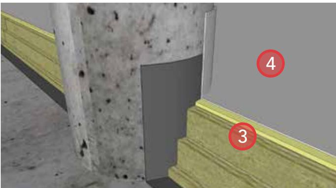
3. Install protection board to provide additional rigidity for the deck surface and protect the insulation below.
