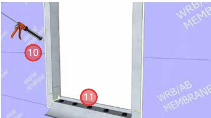
11. Install window shims on the sill of the rough opening.
