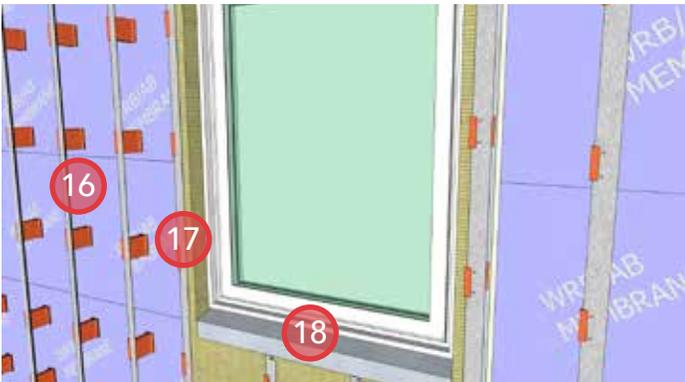
18. Tie in the sub-sill drainage membrane, ensuring that it is positively sloped and fully supported by the ROCKWOOL CAVITYROCK®.
