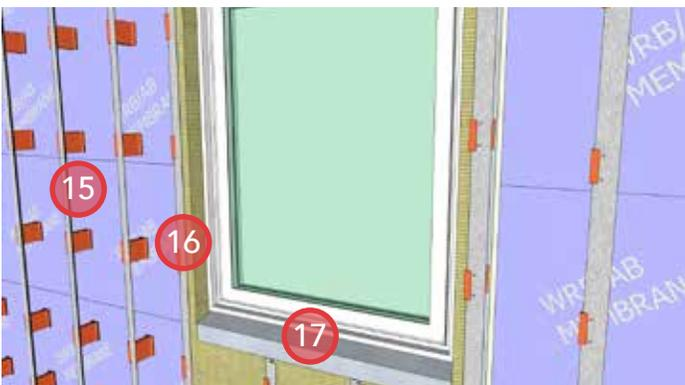
17. Tie in the sub-sill drainage membrane, ensuring that it is positively sloped and fully supported by the ROCKWOOL CAVITYROCK®.
