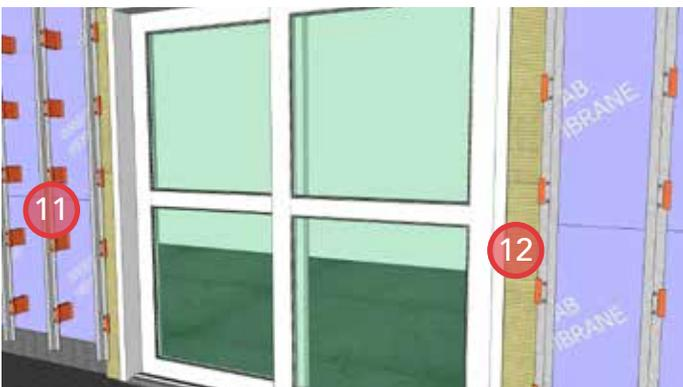
13. Install jamb flashing to aid in future water diversion. Flashing is structurally supported by the girts and provides additional support for ROCKWOOL CAVITYROCK® insulation.
