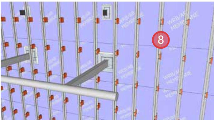
8. Secure clip and rail cladding attachment system to the steel studs per the manufacturer's specifications. Refer to the front end of this guide for further details.
