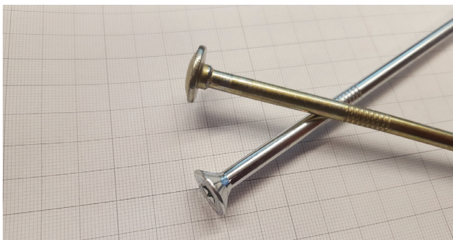
Pan head and counter sunk screws used to attach strapping on the wood-frame backup walls
