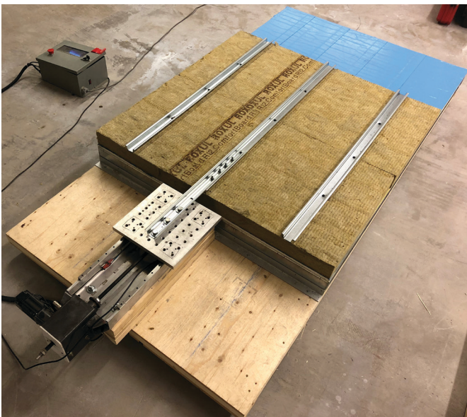
Overview of the strapping load/deflection test apparatus
