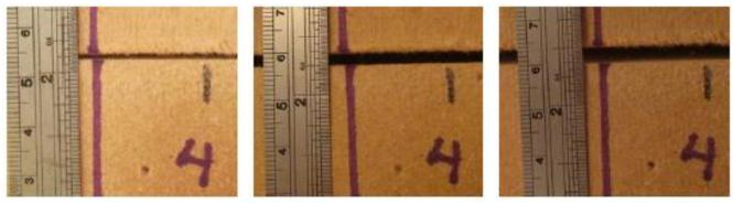
Figure 3: Photographs of measurement location for polyisocyanurate during Phase 2a, cycle #1, #3 and #6 at -18°F (-28°C)
