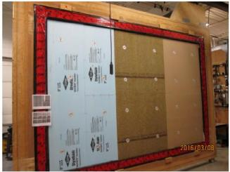
Figure 1: Full scale roof assemblies, Phase 2a (from left: XPS, ROCKWOOL TOPROCK DD, Polyisocyanurate)
