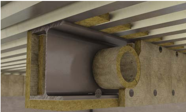
Figure 9 Beam with circular holes (boxed protection - dry joints)
