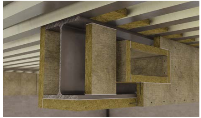
Figure 8 Beam with square or rectangular holes (boxed protection - glued and pinned joints)
